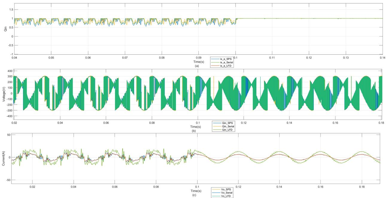
**Figure 14.** Power and output voltage and current waveform. (a) Reactive power waveform, (b) output voltage waveform, (c) input current waveform.
