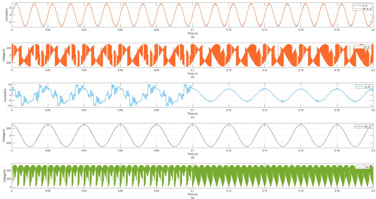
**Figure 3.** SPS offline simulation: (a) output phase A current, (b) output phase A voltage, (c) input phase A current, (d) input phase A voltage, (e) DC bus voltage.
