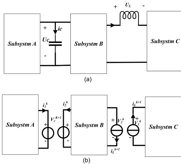
Figure 5. Latency-free decoupling method: (a) before decoupling, (b) after decoupling.
