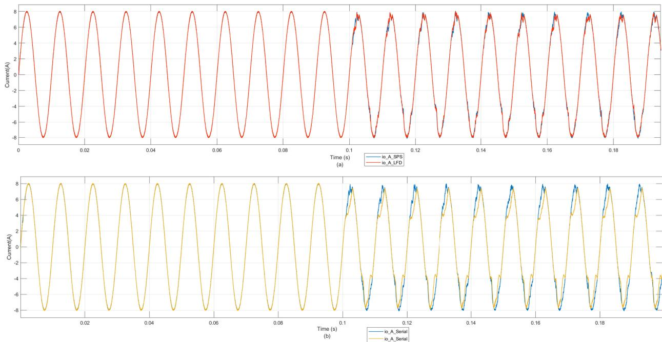
**Figure 12.**  $i_o$  current waveform: (a) SPS-LFD comparison (b) SPS-serial comparison.
