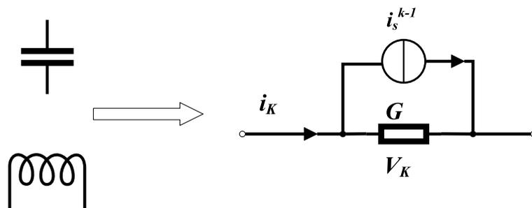
Figure 6. Capacitor-inductor equivalent replacement.
