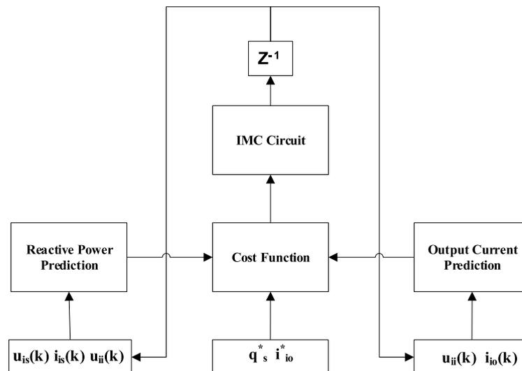
Figure 2. FCS–MPC control flow.
