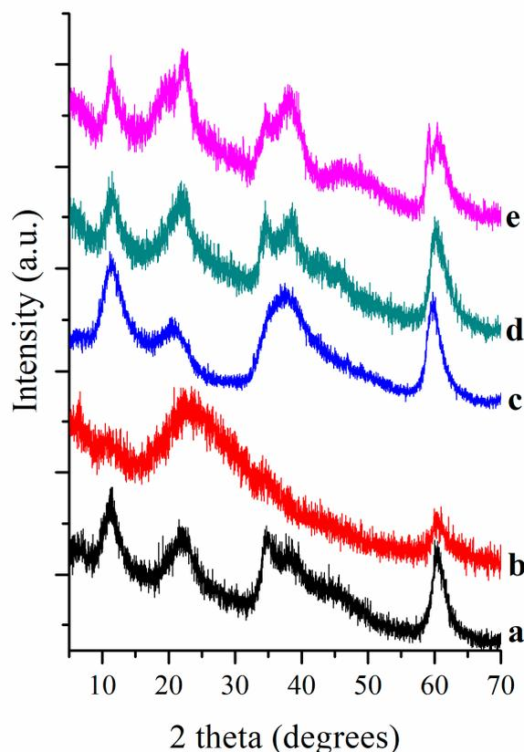
**Figure 1.** XRD patterns of pigments generated by sorption of carminic acid onto layered double hydroxides. (a) LDH-CA, (b) FLDH-CA, (c) FLDH-CA + MgO, (d) ME-FLDH-CA, and (e) ME-FLDH-CA + MgO.
