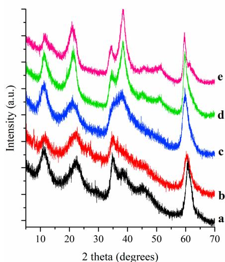
**Figure 5.** XRD patterns of pigments aged for 10 years. (a) LDH-CA, (b) FLDH-CA, (c) FLDH-CA + MgO, (d) ME-FLDH-CA, and (e) ME-FLDH-CA + MgO.
