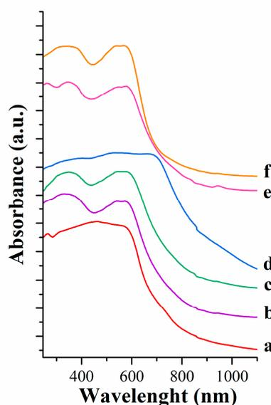
**Figure 4.** UV-vis spectra of carminic acid and pigments generated by sorption of carminic acid onto layered double hydroxides. (a) CA, (b) LDH-CA, (c) FLDH-CA, (d) FLDH-CA + MgO, (e) ME-FLDH-CA, and (f) ME-FLDH-CA + MgO.
