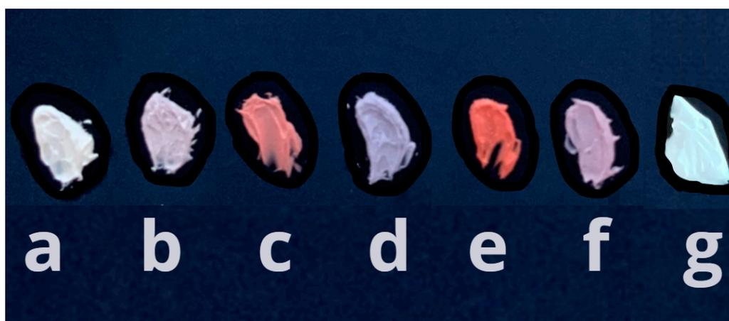
**Figure 7.** Pigmented emollient creams prepared from white cream (a) and several pigments. (b) LDH-CA, (c) FLDH-CA, (d) FLDH-CA + MgO, (e) ME-FLDH-CA, and (f) ME-FLDH-CA + MgO. As a reference, the white pigment made using FLDH is shown in (g).
