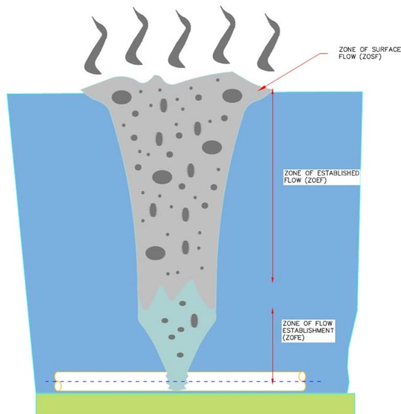
**Figure 3.** Gas Release from a Rupture Subsea Pipeline [43–46].
