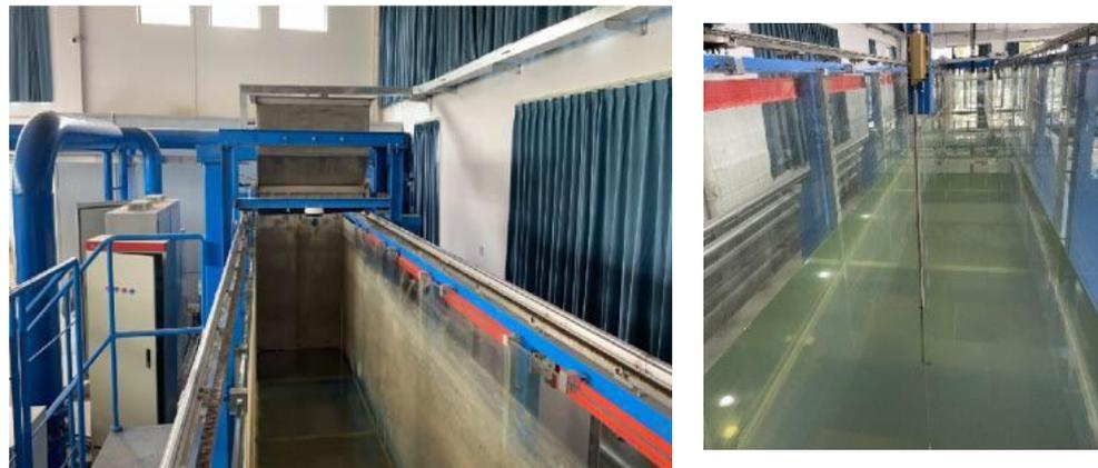
Figure 2. Wave flume.
