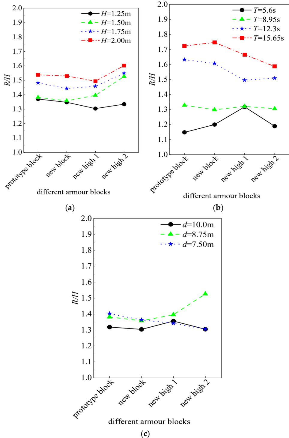
**Figure 11.** Comparison of wave relative run-up for different armor blocks. (a)  $d = 7.5\text{ m}$ ,  $T = 8.95\text{ s}$  (b)  $d = 7.5\text{ m}$ ,  $H = 1.5\text{ m}$ . (c)  $H = 1.5\text{ m}$ ,  $T = 8.95\text{ s}$ .
