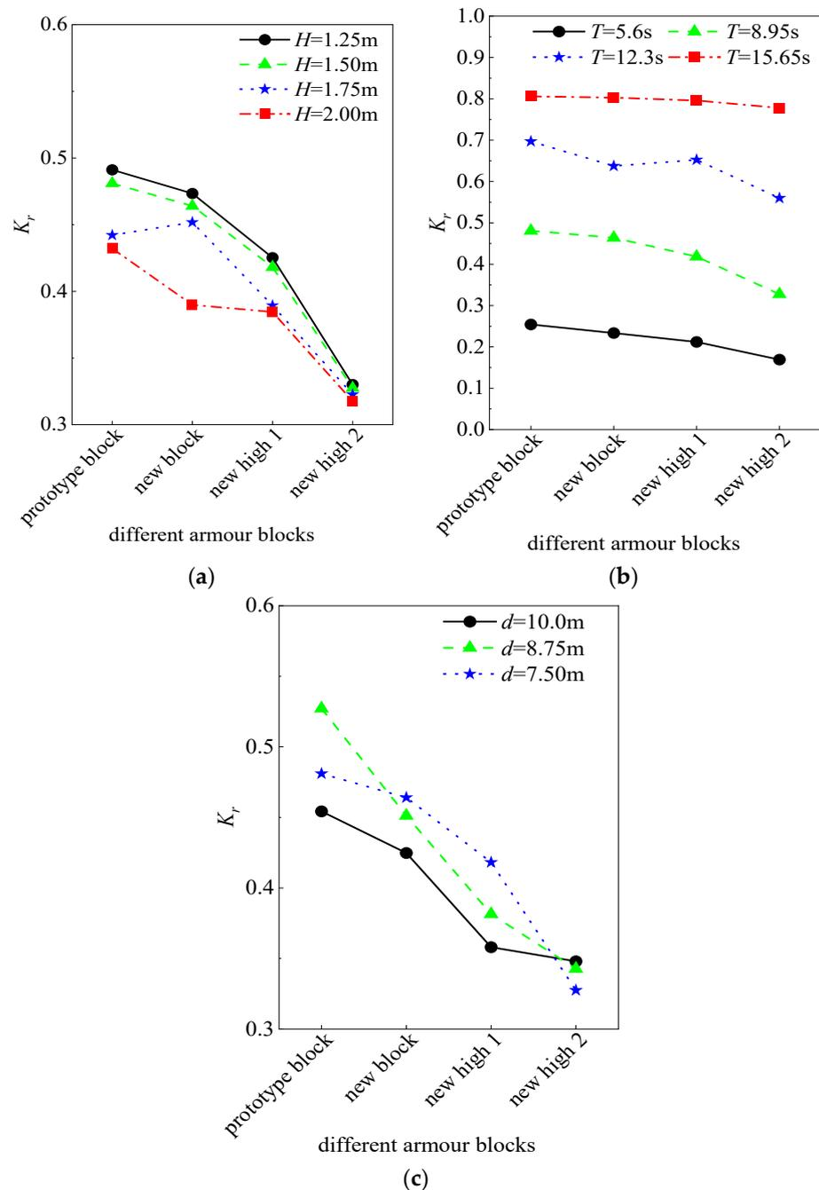
**Figure 10.** Comparison of reflection coefficients for different armor blocks. (a)  $d = 7.5 \text{ m}$ ,  $T = 8.95 \text{ s}$ . (b)  $d = 7.5 \text{ m}$ ,  $H = 1.5 \text{ m}$ . (c)  $H = 1.5 \text{ m}$ ,  $T = 8.95 \text{ s}$ .
