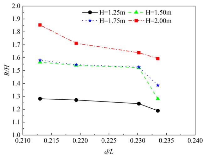
**Figure 9.** The variation in wave run-up with relative water depth at different wave periods.
