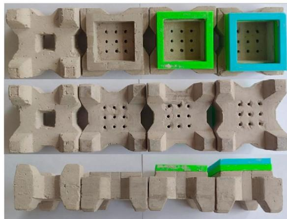
Figure 4. Prototype block and the new block with different frame heights.
