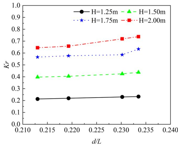
Figure 7. The variation in the reflection coefficient with the relative water depth.
