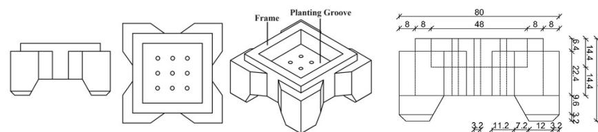
**Figure 1.** Schematic diagram of the new type of ecological quadrilateral hollow block.
