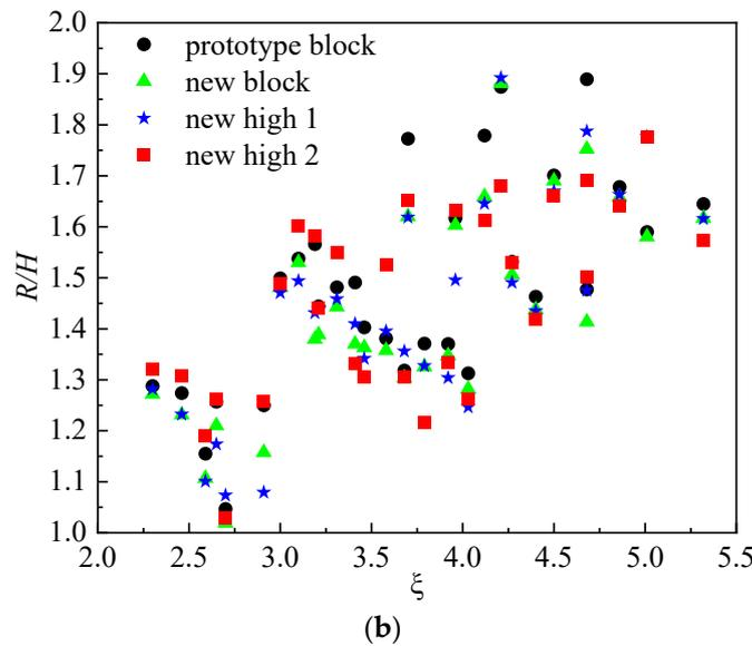
**Figure 12.** The impact of  $\xi$  on reflection coefficient and run-up. (a)  $\xi$  and reflection coefficient  $Kr$ . (b)  $\xi$  and relative run-up  $R/H$ .
