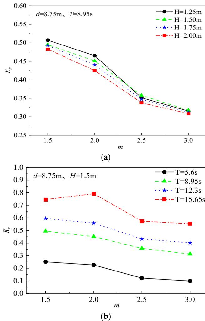
**Figure 6.** The variation in the reflection coefficient with the slope gradient. (a) Effect of slope on reflection coefficients of new blocks under different incident wave height conditions. (b) Effect of slope on reflection coefficients of new blocks under different incident wave period conditions.
