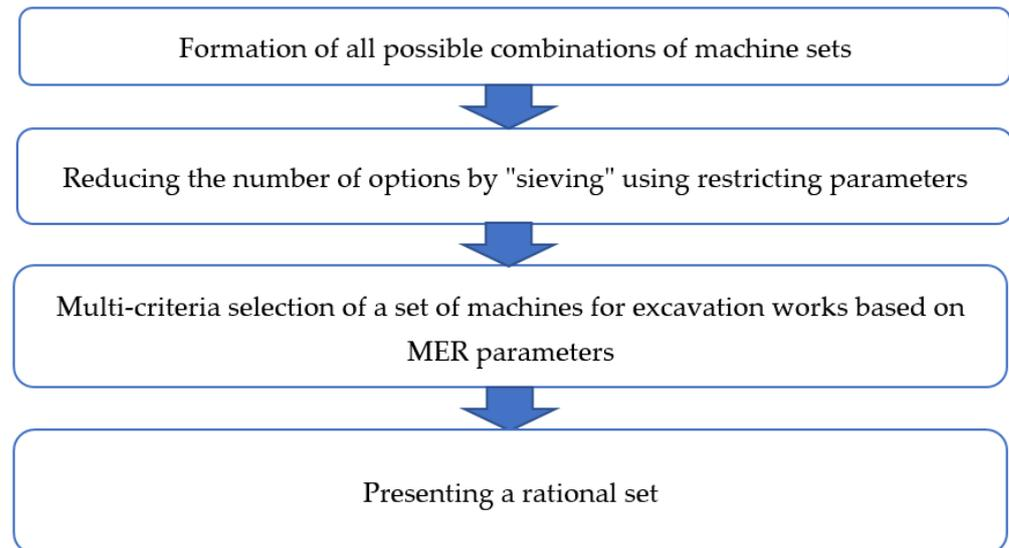
**Figure 1.** The block diagram for selecting a rational set of machines.
