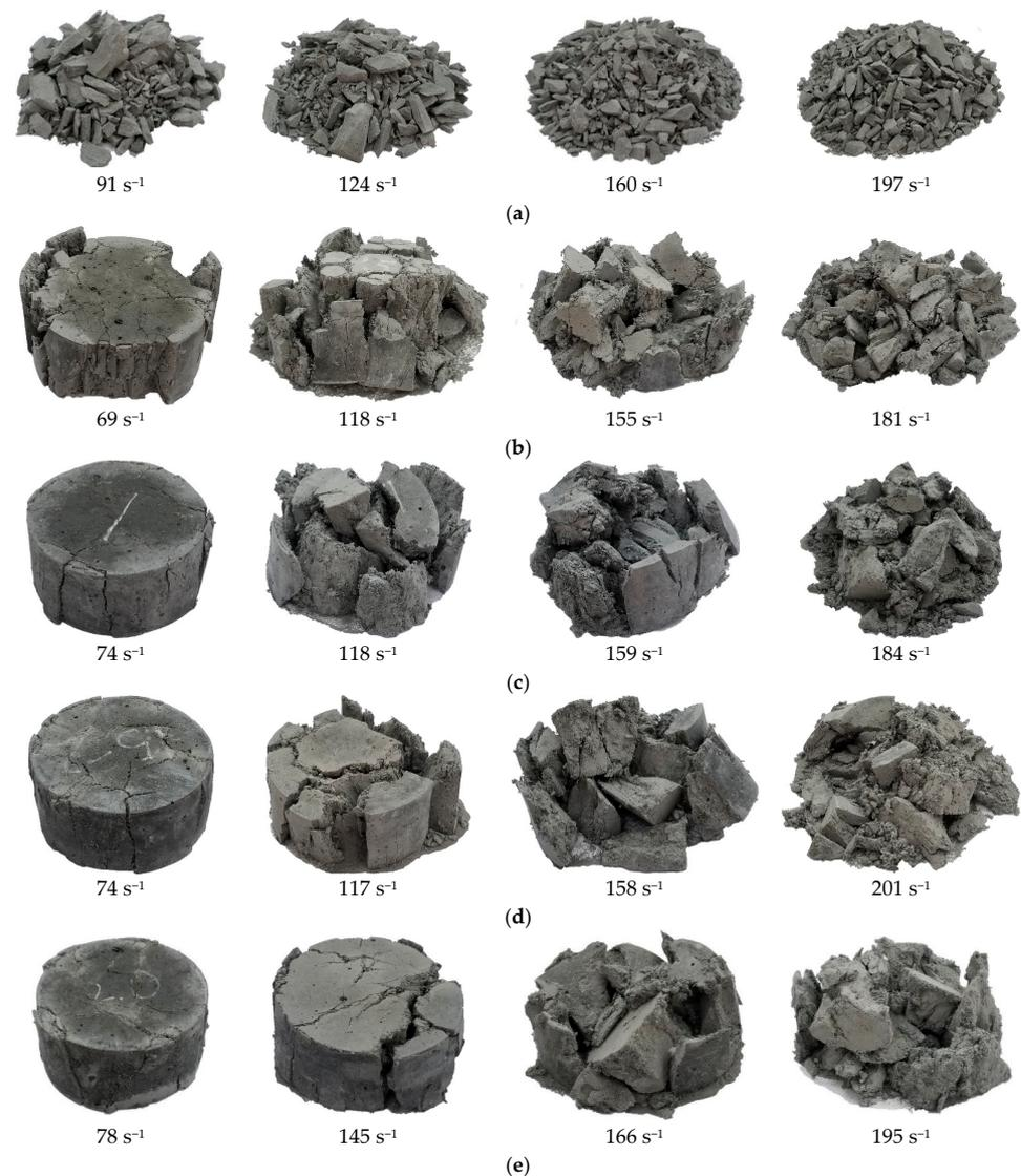
**Figure 14.** Failure patterns of all mixtures under impact loadings: (a) M, (b) PE0.5, (c) PE1.0, (c) PE1.0, (d) PE1.5, (e) PE2.0.
