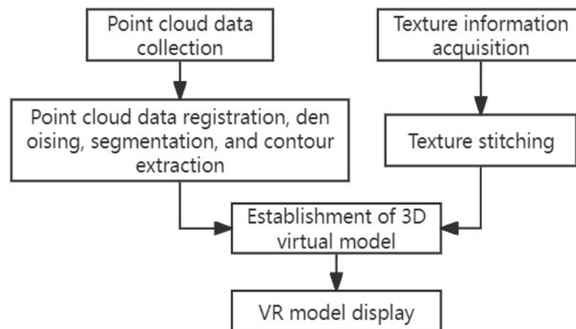
Figure 4. Data processing and modeling flow.
