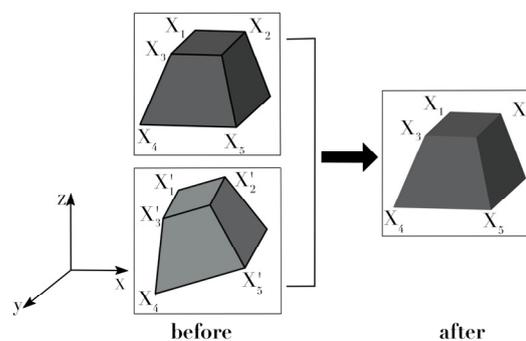
Figure 11. Principle of ICP alignment.
