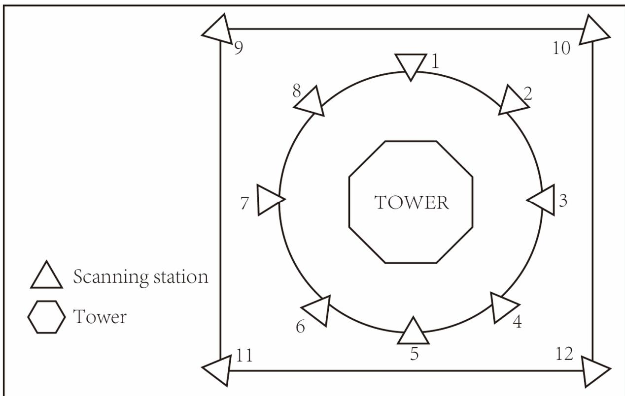
**Figure 8.** Schematic diagram of the scanning point arrangement.
