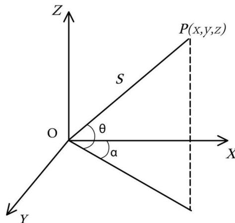
**Figure 7.** Schematic diagram of the spatial coordinate principle of the 3D laser scanner.
