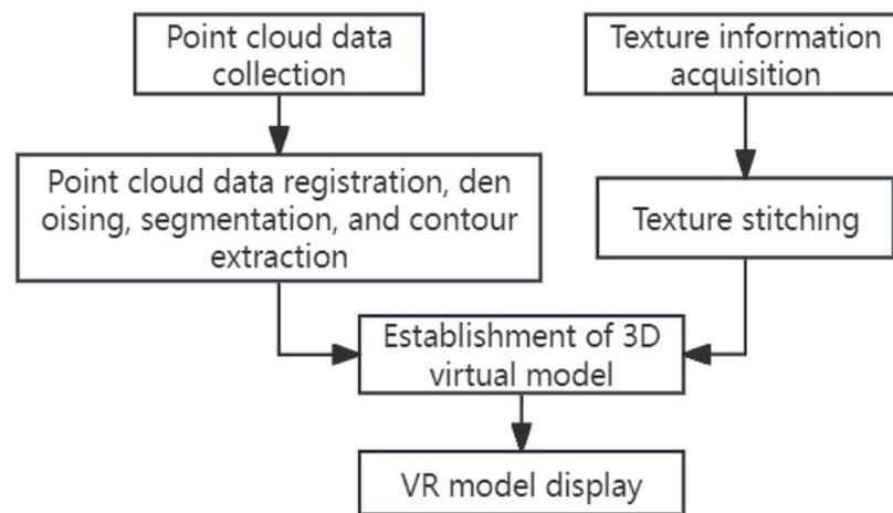
Figure 4. Data processing and modeling flow.
