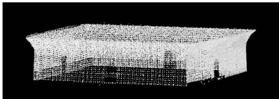
**Figure 13.** Effect of local point cloud block segmentation.
