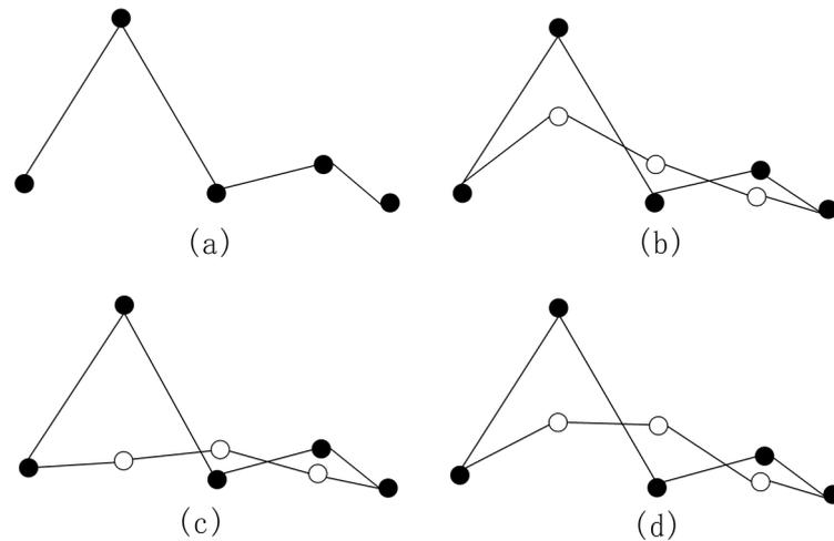
**Figure 12.** Filter processing denoising schematic diagram. (a) Original data. (b) Gaussian filter processing. (c) Mean filter processing. (d) Median filter processing.
