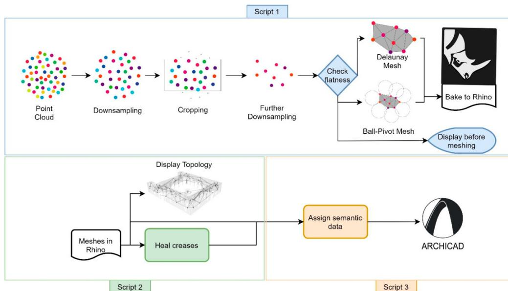
Figure 5. Automatic parameterization workflow [16].
