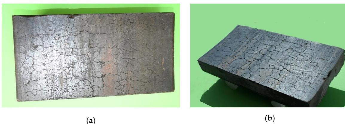
**Figure 4.** Images of brake pad surface: (a) taken perpendicular to its surface; (b) taken from a particular angle that allows us to avoid glares.
