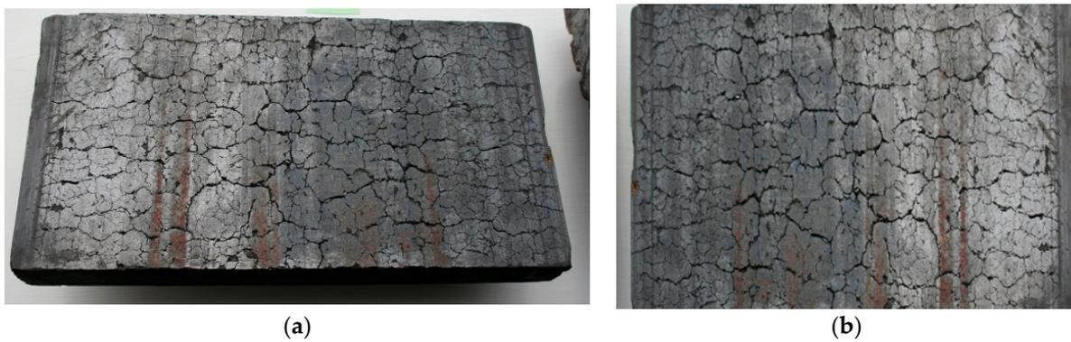
**Figure 12.** Mapping results: (a) obtained image; (b) restored image of the surface of a brake pad.
