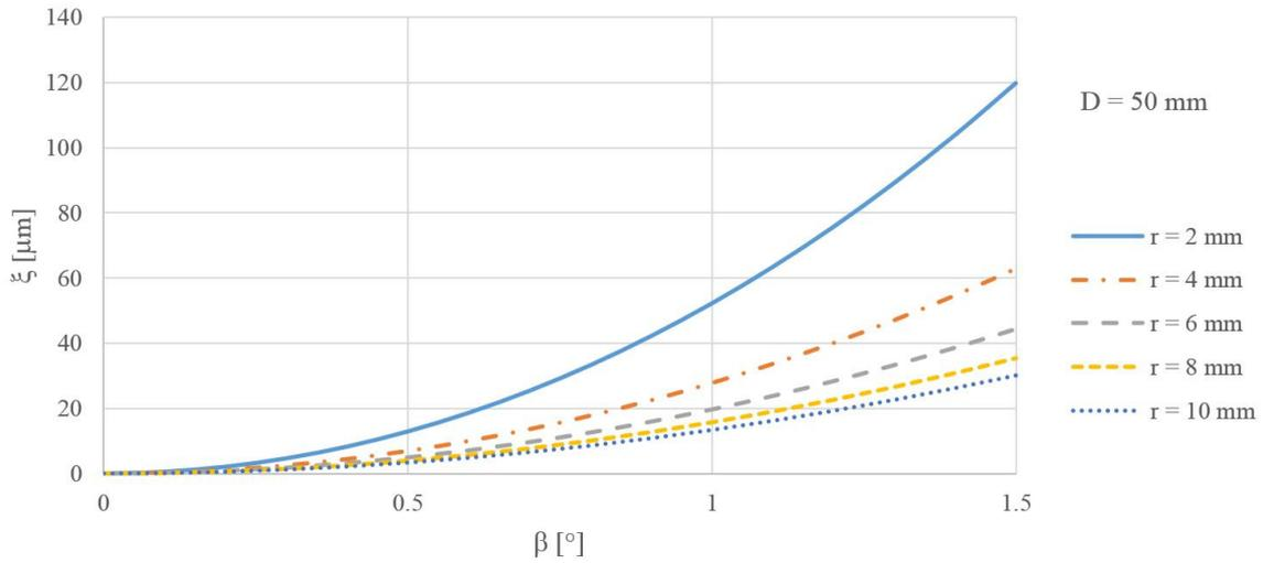
**Figure 5.** The size of the error  $\zeta$  for different tilts  $\beta$  and radii of the forming circle  $r$  of the surface formed by the inner part of the anuloid.
