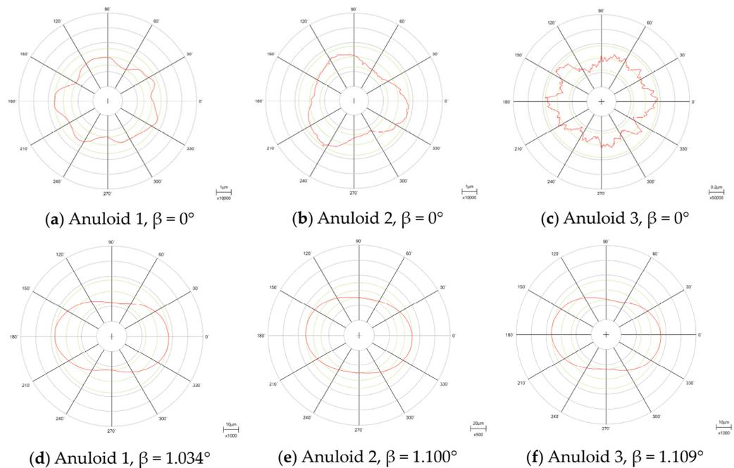
Figure 10. Roundness profiles measured on the surface formed by the inner anuloid ( $\beta$ : inclination angle).
