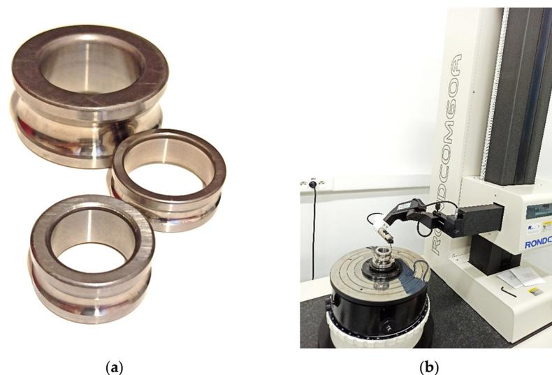
**Figure 9.** Experimental setup: (a) measured parts; (b) round gauge Rondcom 60 A.
