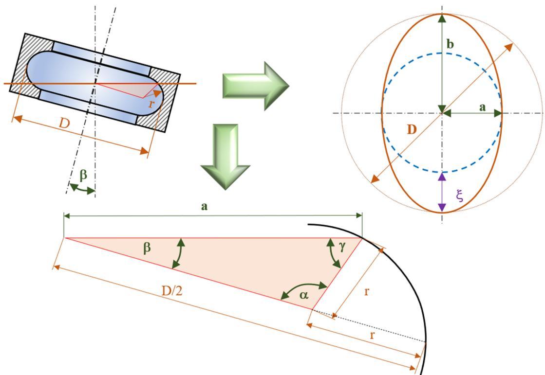
**Figure 6.** Scheme to determine the systematic error of a clamped area formed by the outer part of an anuloid.  $D$ : diameter of the measured anuloid surface;  $r$ : radius of the forming circle;  $a$ : semi-minor axis of the ellipse (roundness profile);  $b$ : semi-major axis of the ellipse (roundness profile);  $\zeta$ : systematic error of the setting.
