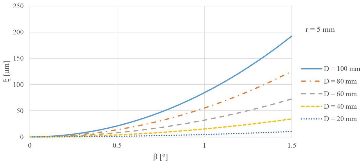
**Figure 4.** The size of the error  $\zeta$  for different tilts  $\beta$  and diameters  $D$  of the area formed by the inner part of the anuloid.
