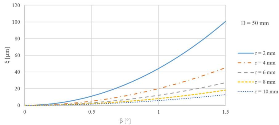
**Figure 8.** The size of the error  $\zeta$  for different tilts  $\beta$  and radii of the forming circle  $r$  of the surface formed by the outer part of the anuloid.
