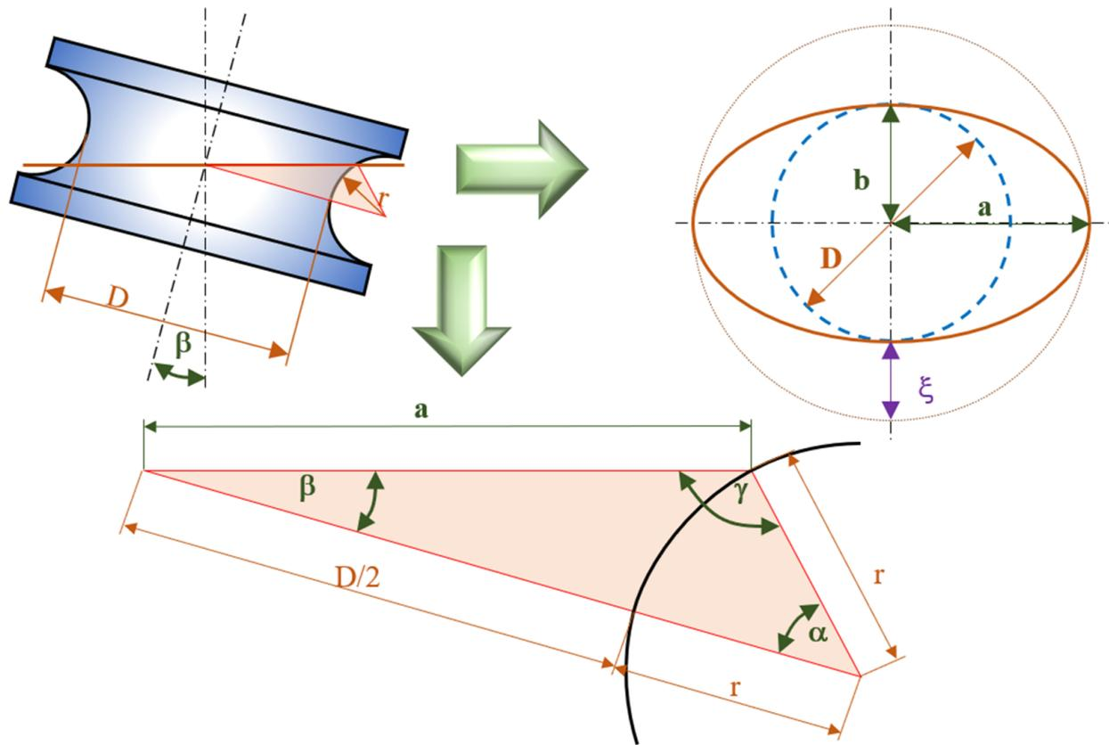
**Figure 3.** Scheme to determine the systematic error of a clamped area formed by the inner part of an anuloid.  $D$ : diameter of the measured anuloid surface;  $r$ : radius of the forming circle;  $a$ : semi-major axis of the ellipse (roundness profile);  $b$ : semi-minor axis of the ellipse (roundness profile);  $\xi$ : systematic error of the setting.
