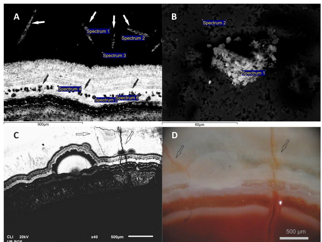
**Figure 6.** SEM micrographs of the Mehane (A,B) and the Rasovača (C,D) vein agate samples. (A) Micrograph (CLI SEM) of Mehane vein agate showing barite inclusions (white arrows) and Fe-oxide inclusions (black arrows) concentrated within the agate band. The barite crystals are largely
