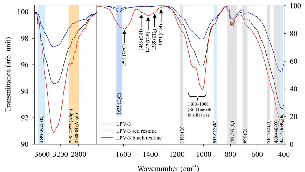
**Figure 10.** FTIR spectra of LPV-3 nodular agate and the incrustation lining cavity in geode from the Lece Volcanic Complex. Red and black residues are attributed to incrustation (explained in text). The left pane illustrates the OH-region and aliphatic organic component regions (3800–2600 cm<sup>-1</sup>), while the right pane displays the fingerprint region of (1800–400 cm<sup>-1</sup>). Abbreviations: Q—quartz, K—kaolinite, Fls—feldspar, Aliph—aliphatic component.
