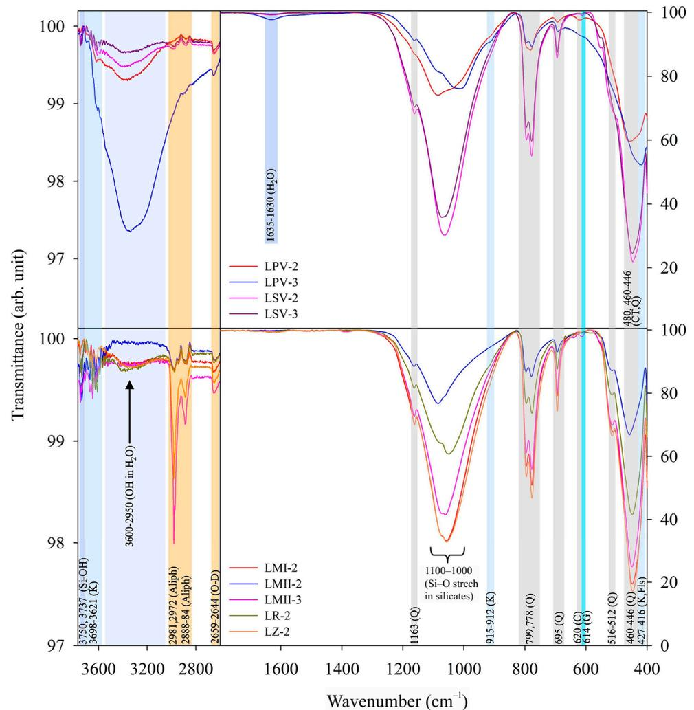
**Figure 9.** FTIR spectra of agate samples from the Lece Volcanic Complex. The OH-region and aliphatic organic component regions ( $3800\text{--}2600\text{ cm}^{-1}$ ) are shown in the left pane, while the fingerprint region ( $1800\text{--}400\text{ cm}^{-1}$ ) is shown in the right pane. Abbreviations: Q—quartz, K—kaolinite, G—goethite, Fls—feldspar, CT—opal, C—cristobalite, Aliph—aliphatic component.
