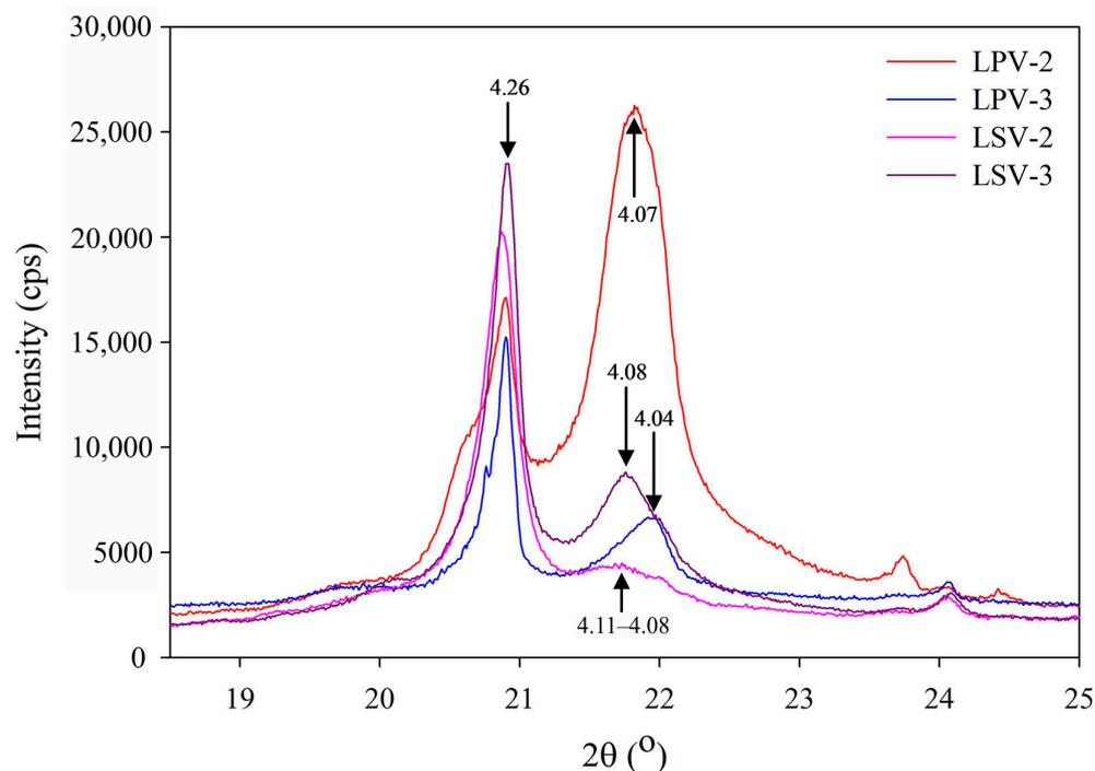
**Figure 8.** XRD pattern of nodular agate samples from the Lece Volcanic Complex. The complex reflection consists of 4.26 Å pertaining to quartz and CT-opal reflection in the range of 4.11–4.04 Å. Agate samples reveal a shift in the opal reflection position indicating variation of  $\alpha$ -cristobalite and  $\alpha$ -tridymite portion in the opal stacking sequence.
