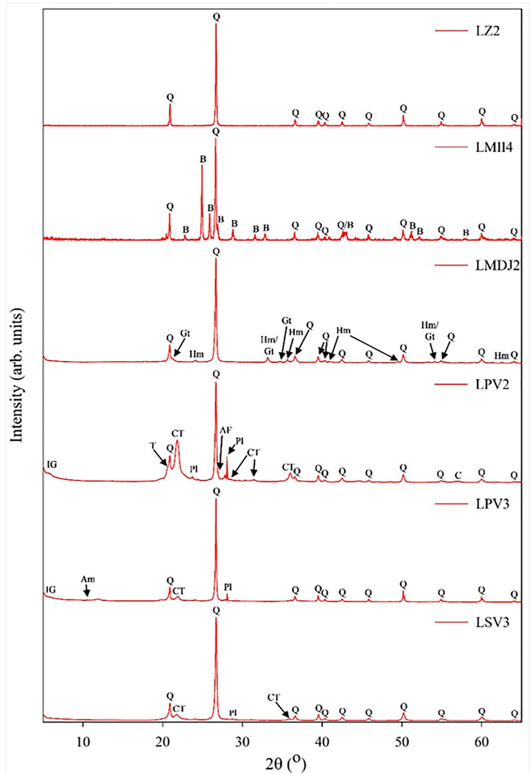
**Figure 7.** XRD pattern of agate samples from the Lece Volcanic Complex. LZ2 and LMII4 are veined agates while the others are nodular agates. Abbreviations: Q—quartz, IG—interstratified clay, CT—opal-CT, B—barite, Hm—hematite, Gt—goethite, Pl—plagioclase, AF—alkali feldspar, Am—amphibole.
