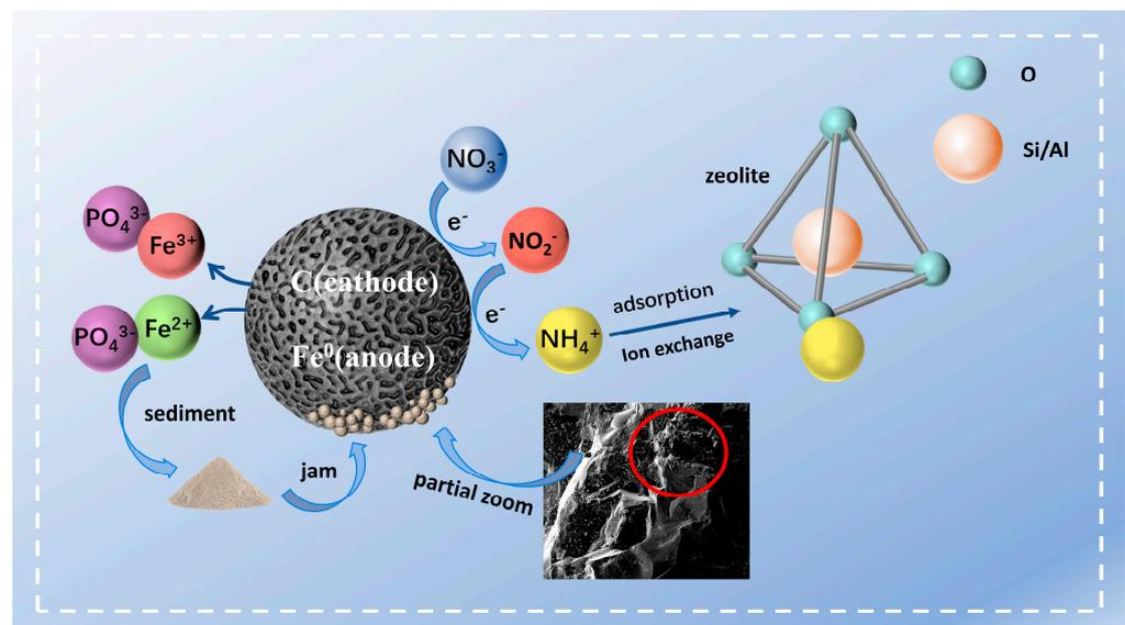
**Figure 8.** Schematic mechanism of phosphate and nitrogen removal by sponge iron and zeolite.
