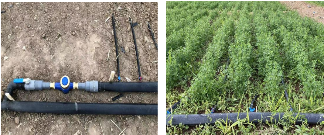
Figure 1. The photo shows the underground drip irrigation system used for water control in each plot of the test plot, which forms alternating irrigation on both sides of the crops by opening and closing the adjacent red and blue bypass valves.
