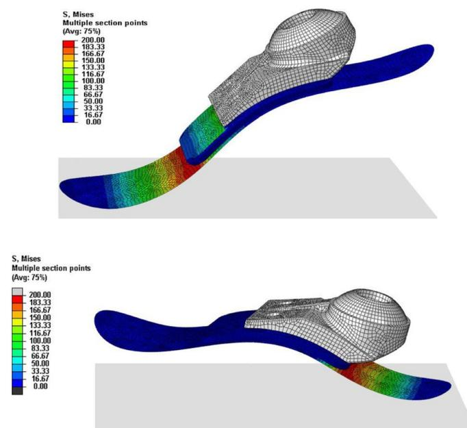
**Figure 8.** Illustrative finite-element analysis of a prosthetic foot designed and studied by Song et al. [164] (Note: The data shown in this figure is for illustrative purposes only and is not relevant to the present discussion). Reproduced with permission from Youngnam Song et al., *International Journal of Precision Engineering and Manufacturing*; published by Springer Nature, 2019.
