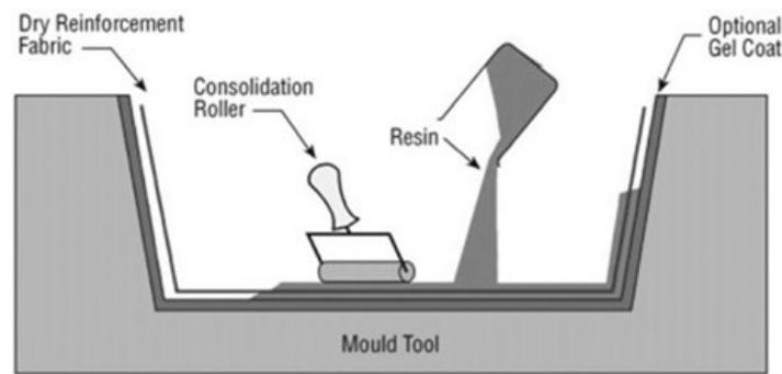
**Figure 3.** Hand-layup method for manufacturing composite materials [145]. Reprinted from *Comprehensive Composite Materials*, Author(s): D. Cripps, T.J. Searle, J. Summerscales, Title of chapter: *Comprehensive Composite Materials*, Pages 737–761, Copyright (2000), with permission from Elsevier.
