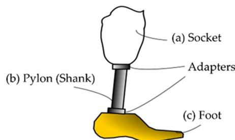
**Figure 1.** Main components of a passive transtibial prosthesis: (a) the socket, the part of the prosthesis that fits over the residual limb (the remaining part of the amputated leg); (b) the shank (or pylon), a rigid component that extends from the socket down to the foot; (c) the foot, the component of the prosthesis that mimics the function of a natural foot, absorbs shock during walking, and provides stability. Reprinted from ref. [58].
