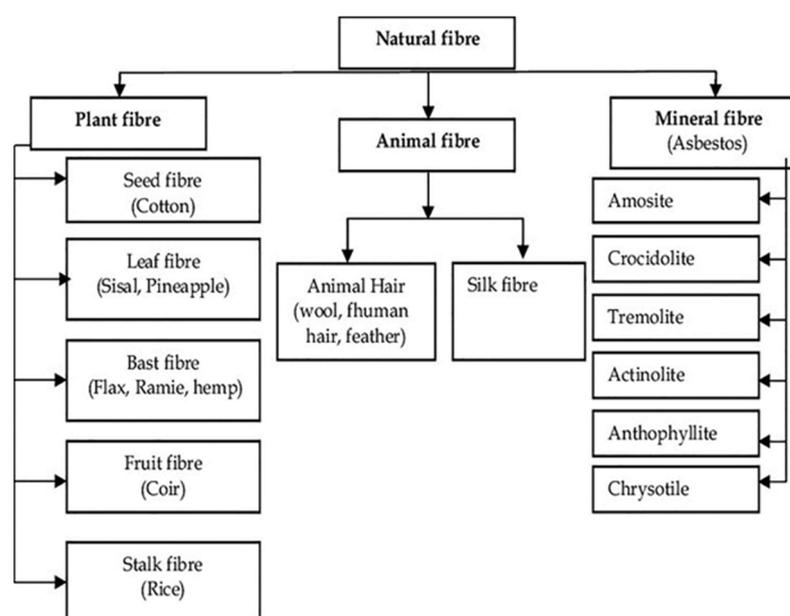
**Figure 2.** Classification of natural fibers based on their origin: plant, animal, or mineral [29]. Reprinted from *Materials Today: Proceedings*, Vol. 50, Sandeep Kumar, Alakesh Manna, Rakesh Dang, A review on applications of natural fiber-reinforced composites (NFRCs), Pages 1632–1636, Copyright (2022), with permission from Elsevier.
