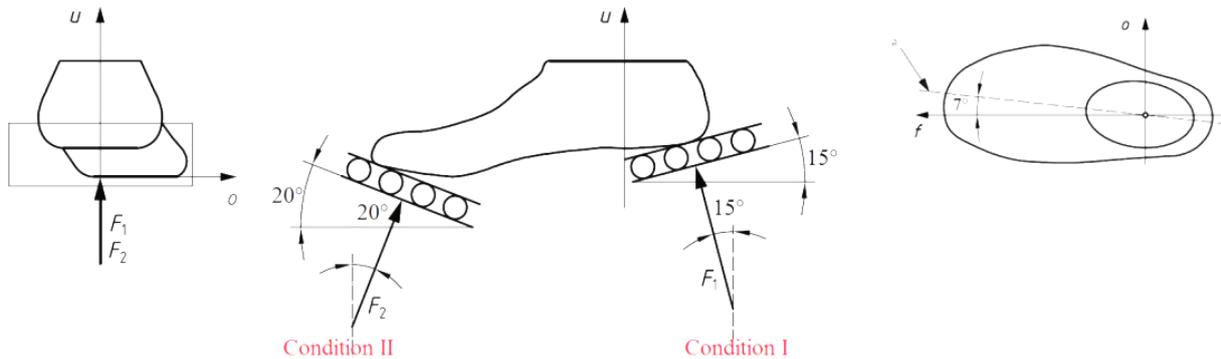
**Figure 6.** Alignment and angles of test loads for a prosthetic foot, established by ISO 10328 [157]. Reprinted from *Procedia Engineering*, Vol. 10, C. Colombo, E.G. Marchesin, L. Vergani, E. Boccafogli, G. Verni, Study of an ankle prosthesis for children: adaptation of ISO 10328 and experimental tests, Pages 3510–3517, Copyright (2011), with permission from Elsevier.
