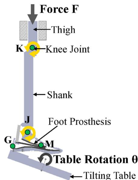
**Figure 7.** Alignment and angles of test loads for a prosthetic foot established in ISO 22675. Reprinted from ref. [158].
