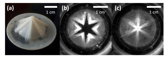
**Figure 2.** (a) Printing result of TIPI 3.4 after removal of the support material. (b) Opened and (c) closed stages within the hemodynamic testing device. The scale bars refer to each individual picture.
