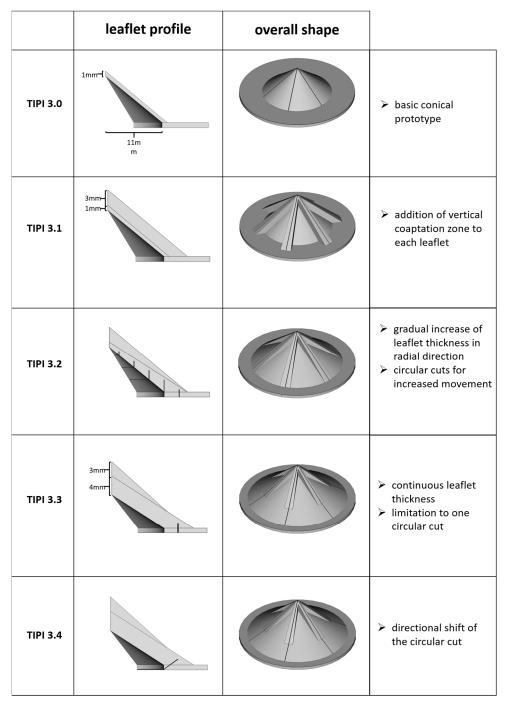
**Figure 1.** Illustration of the different mentioned prototypes, including the profile of a single leaflet (middle column) as well as the overall prototype shape (right column). The metal restrictor structure included in TIPI 3.0 and 3.1, as presented in our previous work, is not shown.
