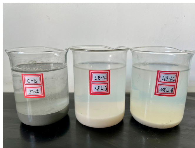
Figure 22. The grouting off target characteristics of C-S and LiB-AC grout.
