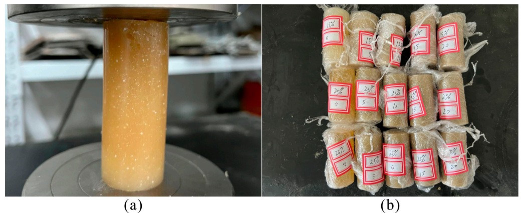
Figure 7. Compressive strength test of LiB-AC grout: (a) the process of compressive strength test; (b) specimens for compressive strength test.
