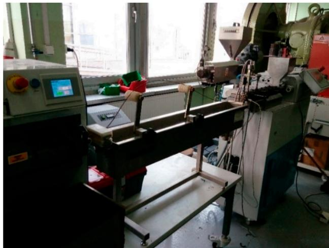
**Figure 1.** Extrusion line using ZAMAK REA-2P12A Explorer twin-screw extruder used to extrude the PHBV-hemp fiber and PHBV-flax-fiber biocomposites.
