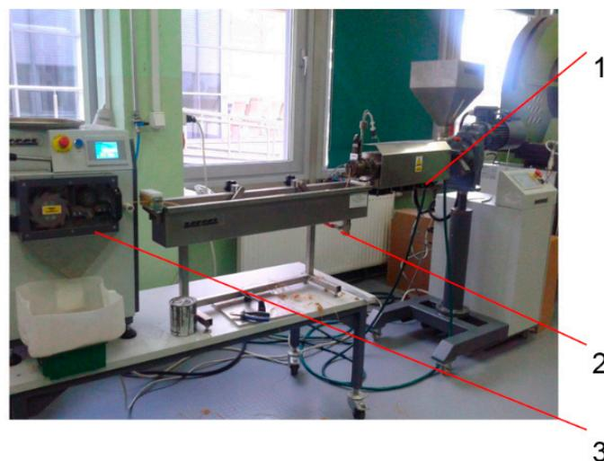
**Figure 3.** The extrusion line of PHBV- plant origin fiber biocomposites: 1—ZAMAK EHP-25E extruder, 2—cooling bath, 3—granulators.
