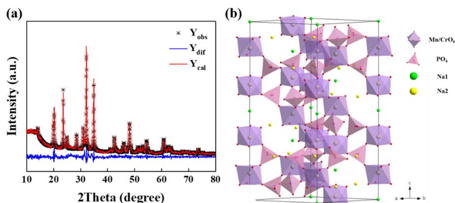
**Figure 2.** (a) X-ray diffraction (XRD) and corresponding Rietveld refinement results of NMCP/rGO; (b) crystal structural of NMCP and the coordination of cations.
