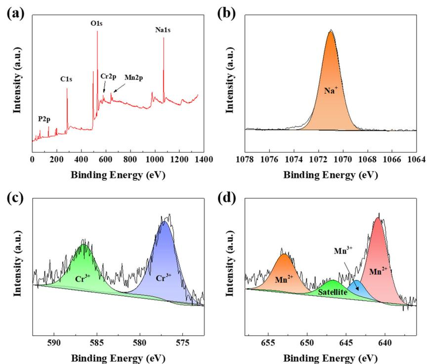
**Figure 5.** XPS spectra of (a) survey, (b) Na 1s, (c) Cr 2p, and (d) Mn 2p of NMCP/rGO.
