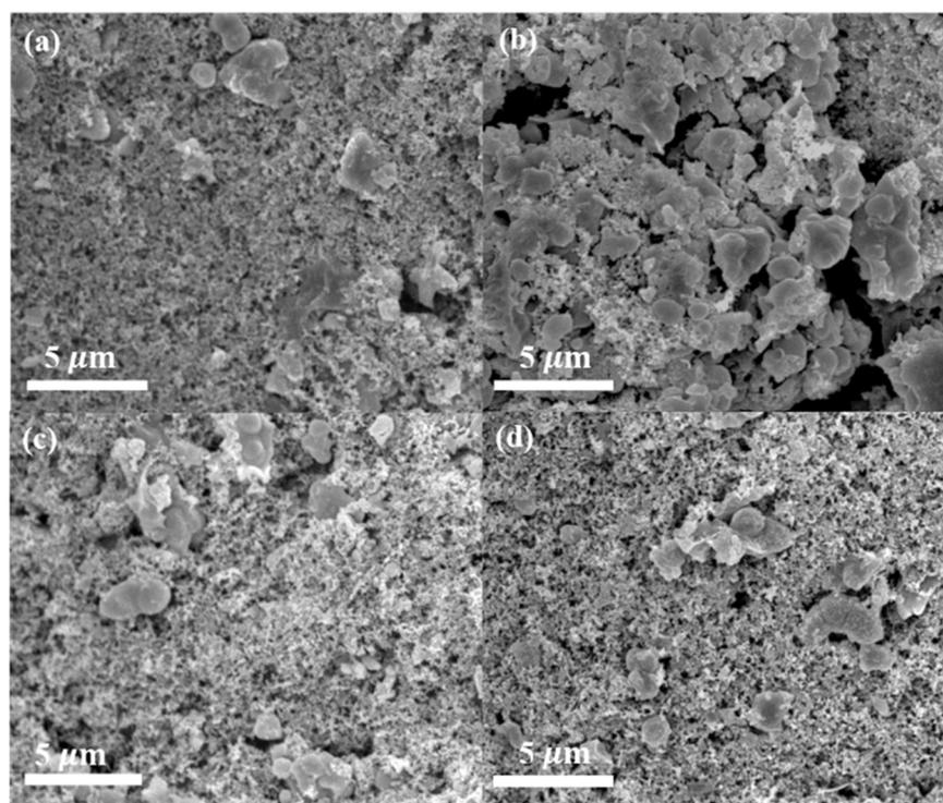
**Figure 10.** SEM images of the cathode before and after cycling. (a) NMCP cathode before cycling; (b) NMCP cathode after cycling; (c) NMCP/rGO cathode before cycling; (d) NMCP/rGO cathode after cycling.
