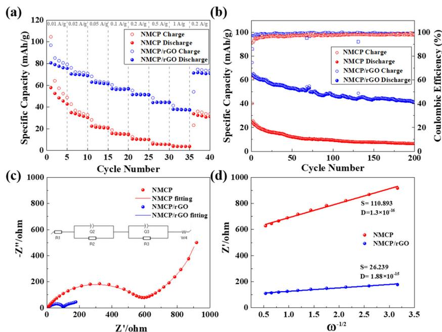
**Figure 8.** NMCP and NMCP/rGO (a) C-rate tests at 0.01 A/g to 1 A/g, (b) cycling performances at 0.1 A/g, (c) Nyquist plots along with the fitting curves and equivalent circuit, and (d) linear relationships between  $Z'$  and the reciprocal square root of angular rate ( $\omega^{-1/2}$ ) in the low frequency region.
