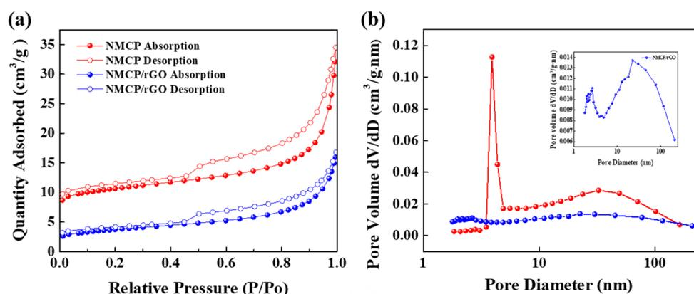
**Figure 6.** Bare NMCP and NMCP/rGO: (a) absorption and desorption isotherms; (b) pore size distributions. Inset in (b) shows the pore size distribution of NMCP/rGO in large magnitude.
