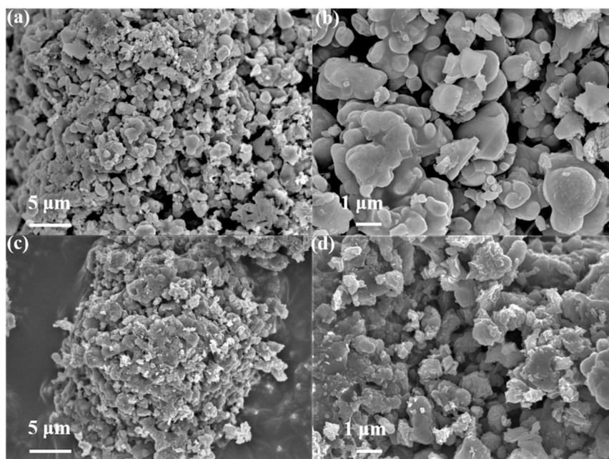
**Figure 3.** SEM images of (a,b) pristine NMCP and (c,d) as-synthesized NMCP/rGO under different magnifications.
