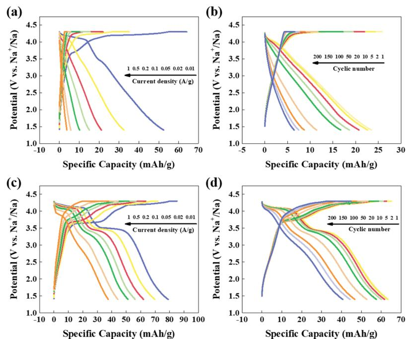
**Figure 9.** (a) Galvanostatic charge/discharge curves of the NMCP electrode at different current rates from 0.01 to 1 A/g. (b) Representative charge/discharge curves of NMCP at 0.1 A/g. (c) Galvanostatic charge/discharge curves of the NMCP/rGO electrode at different current rates from 0.01 to 1 A/g. (d) Representative charge/discharge curves of NMCP/rGO at 0.1 A/g.
