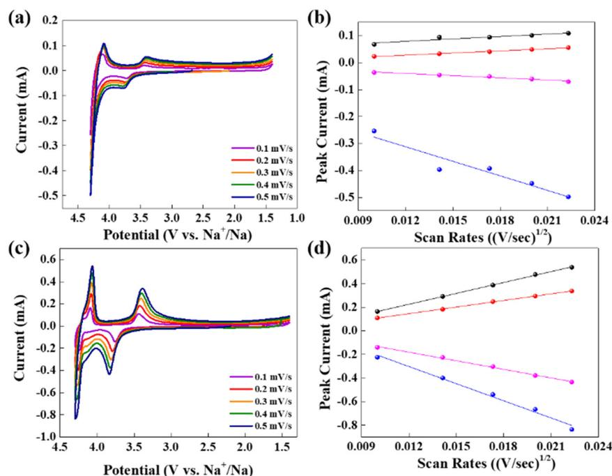
**Figure 7.** Cyclic voltammograms profiles of (a) NMCP and (c) NMCP/rGO at 0.1 mV/s to 0.5 mV/s, and the relationship between the peak currents and the square root of the scan rates of (b) NMCP and (d) NMCP/rGO.
