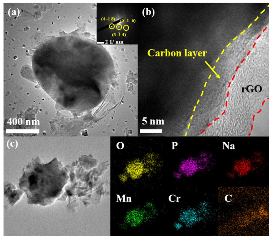
**Figure 4.** (a,b) TEM images of NMCP/rGO and SAED; (c) NMCP/rGO elemental mappings of oxygen (yellow), phosphorus (purple), sodium (red), manganese (green), chromium (blue) and carbon (orange).
