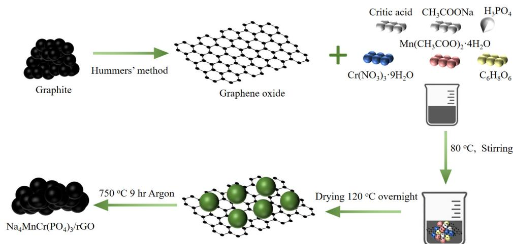
**Figure 1.** Illustrations of the Hummers' method and the sol-gel process for preparing  $\text{Na}_4\text{MnCr}(\text{PO}_4)_3$ .
