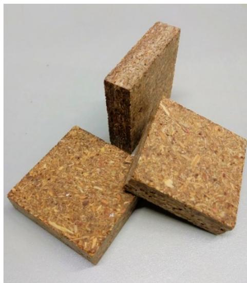
**Figure 10.** PB samples (5 cm × 5 cm) manufactured with 13.2% binder solids relative to the dry wood particles and pressed at 190 °C for 10 min.
