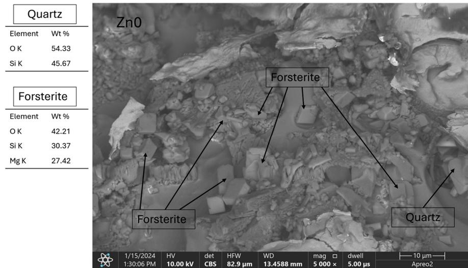
Figure 4. Microstructure of Zn0 glazes at 5000× magnification with EDS analysis.
