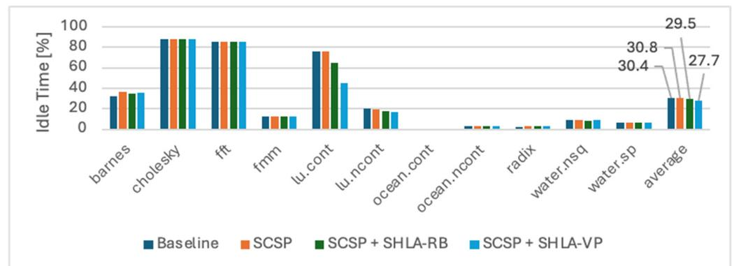
**Figure 13.** Idle time for each benchmark using multiple microarchitectural configurations (16 cores).
