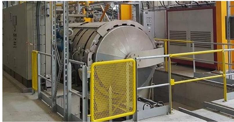
Figure 2. Autoclave for carbonation at the Orbix pilot facilities.
