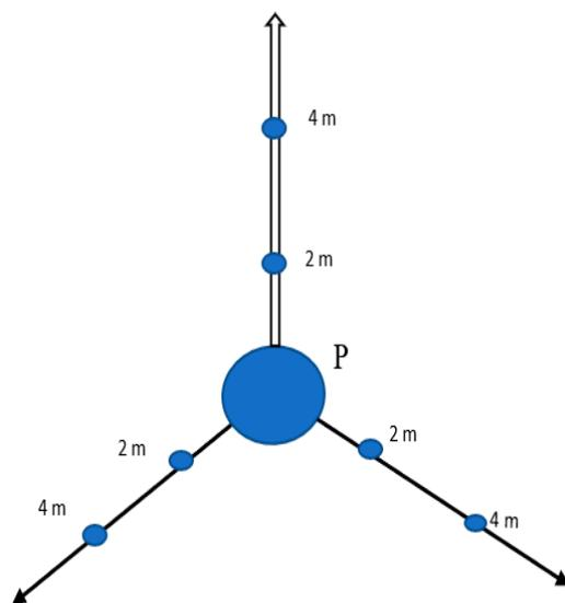
**Figure 3.** Approach used when sampling soils from metal fabrication workshops in Mbarara City, Uganda.
