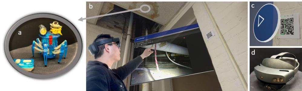
**Figure 16.** (a) HEXBUG Spider located in confined ceiling space, (b) human wearing AR headset with inset showing first-person view from the microrobot, (c) QR code detected in AR headset, (d) AR headset used to inspect the damaged pipe.
