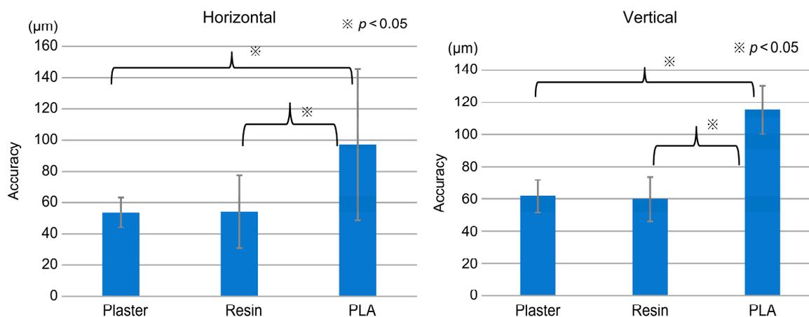
**Figure 3.** Comparison of the horizontal and vertical accuracies of the three models. We can observe significant differences in both horizontal and vertical accuracies between plaster and poly(lactic acid) (PLA) and resin and PLA.
