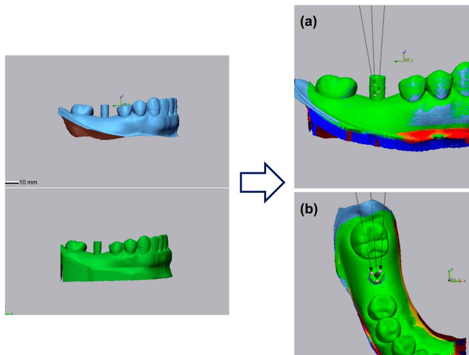
**Figure 2.** Stereolithography (STL) of the base model superimposed on each of the models to measure accuracy. For horizontal and vertical accuracies, three points were randomly selected, and their average was used as the result. (a) Horizontal and (b) vertical accuracy.
