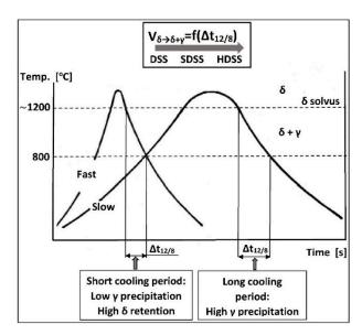
**Figure 6.** Influence of cooling rate on the content of δ-ferrite in duplex steels (according to [30]). Left-hand frame: fast cooling, high δ-ferrite content; right-hand frame: slow cooling, high content of  $\gamma$ -austenite precipitates.
