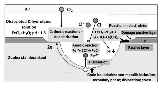
**Figure 11.** Pitting corrosion mechanism of duplex steel when exposed to chloride attack (according to [21]).
