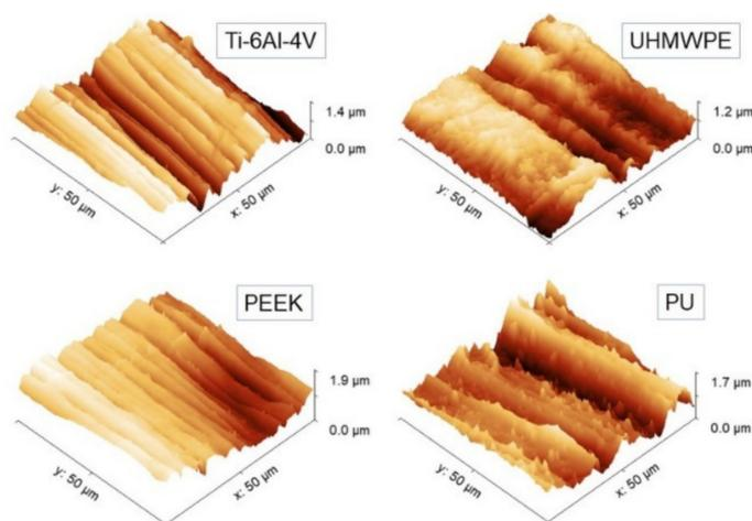
**Figure 3.** Representative  $50 \times 50 \mu\text{m}^2$  AFM topographies of the four surfaces investigated. All the images have been displayed at the same rotation angle for a guide to the eye.
