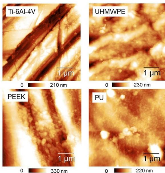
**Figure 6.**  $5 \times 5 \mu\text{m}^2$  AFM topographies of the four surfaces.
