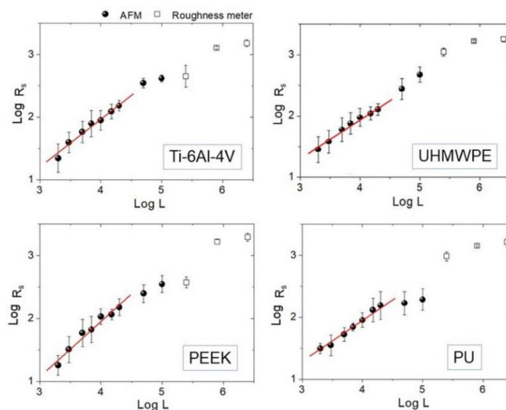
**Figure 4.** Log-Log plots of  $R_s$  vs.  $L$  curve for each sample. Experimental points measured by AFM (black round dots) and roughness meter (square dots) are reported together. Linear fittings on AFM data below  $L = 20 \mu\text{m}$  are also highlighted.
