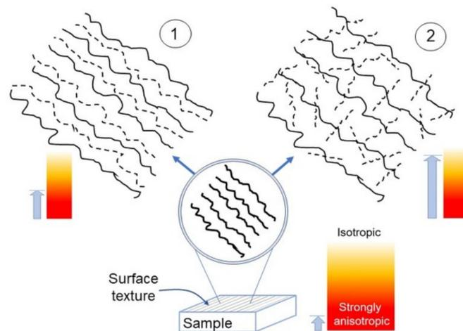
**Figure 8.** Sketch of the anisotropy appearance in a surface possessing a single lay (bottom), upon magnification in the case 1 (top left) and 2 (top right). The light blue arrows roughly indicate the corresponding anisotropy strength.
