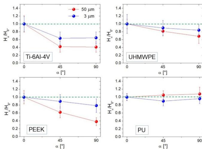
**Figure 7.**  $H_\alpha/H_{0^\circ}$  ratios for  $\alpha = 45^\circ$  and  $90^\circ$  calculated at  $L = 50$  (red curve) and  $3 \mu\text{m}$  (blue curve). The green dotted lines indicate unity (full isotropy) for the reader's convenience.
