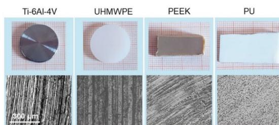
**Figure 1.** The four materials used in this work (**top**) and (**bottom**) corresponding  $20\times$  optical images of their surfaces. The scale bar on the left is the same for all the images.
