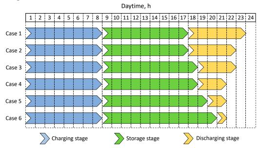
Figure 6. Daily operating plan of different variants of the A-CAES system.
