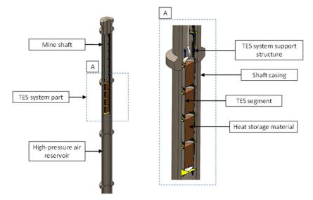
Figure 3. The structure of the TES installation located in the post-mine shaft.
