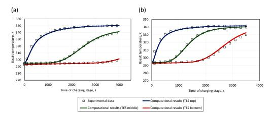
**Figure 5.** Experimental and numerical results of the TES tank charging process: (a)  $T_{max} = 350.25$  K, (b)  $T_{max} = 341.75$  K.
