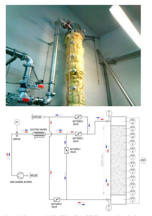
**Figure 4.** Laboratory stand of the TES installation [27]. The arrows indicate the direction of flow: (red) hot air, (blue) cold air. Copyright (2022), with permission from Elsevier.
