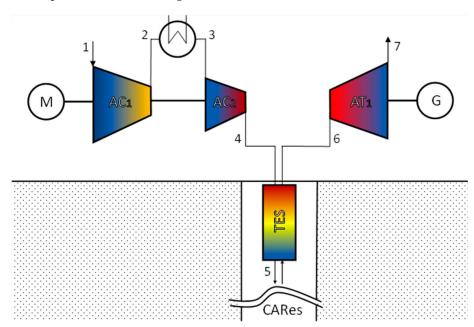
Figure 2. Schematic of the adiabatic compressed air energy storage system.
