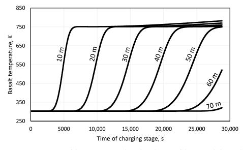
**Figure 7.** Temperature of the storage material at selected points of the TES tank during the charging stage of the system.
