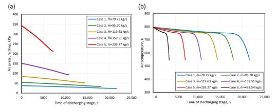
**Figure 8.** The value of (**a**) air pressure drop and (**b**) air temperature during the discharge stage of the A-CAES system.
