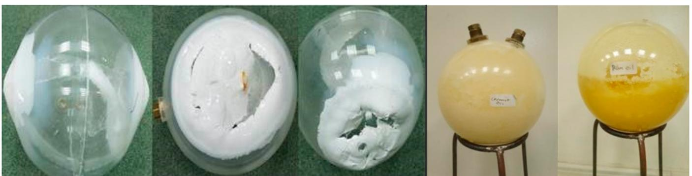
Figure 16. The effect of alcohol on acrylic material and the frozen coconut palm oil at lab temperature.
