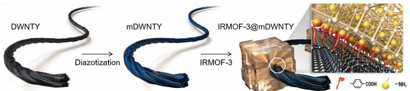
**Figure 18.** Schematics illustrating the synthesis process used to fabricate IRMOF3@mDWNTY (IRMOF3 = ligand-based isorecticular metal-organic framework; mDWNTY = modified double-walled nanotube yarn). Reprinted with permission from [94].
