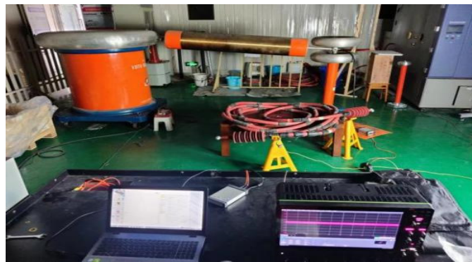
Figure 1. PD test platform for high-speed EMU cable terminals.
