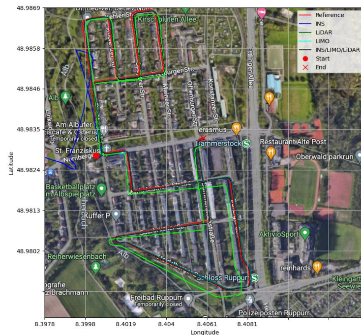
Figure 17. Comparison of trajectories, D-28 (INS/LIMO/LiDAR).
