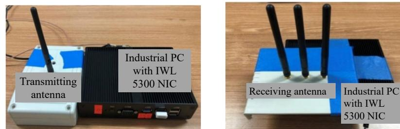
**Figure 6.** CSI data collection equipment. The mobile terminal has a transmitting antenna (left) and the fixed terminal has three receiving antennas (right).
