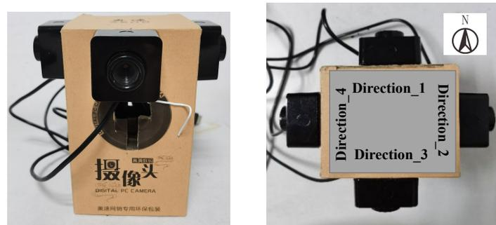
**Figure 7.** Multi-directional images collection equipment. ((Left): front view, (Right): top view).
