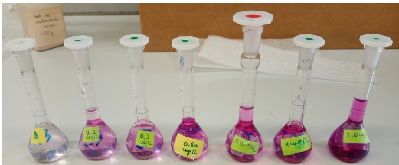
Figure S8. NO 2 - standard solutions (STD1-STD6) in the concentration range (0.2-2 mg/L; 0.0043-0.0435 mM) and blank (B) reacted with Griess reagent system (GRS) and used to construct the calibration curve shown in Figure S9.
