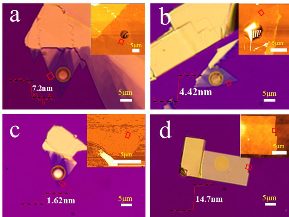
Figure S3. Optical imaging and AFM height profiles of suspended few-layered PdSe<sub>2</sub>. The red rectangles represent the AFM measurement areas, and the red curves represent the height profile.
