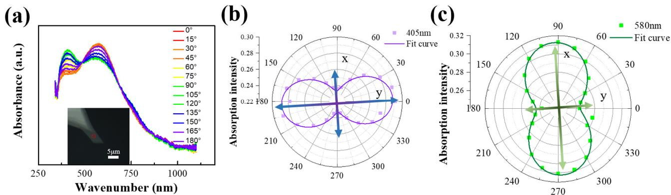
Figure S2. (a) Polarized light absorption spectrum shows the relationship between absorption intensity and polarization angle. (b) and (c) are polarization diagrams of light absorption at 405 and 580nm, respectively.
