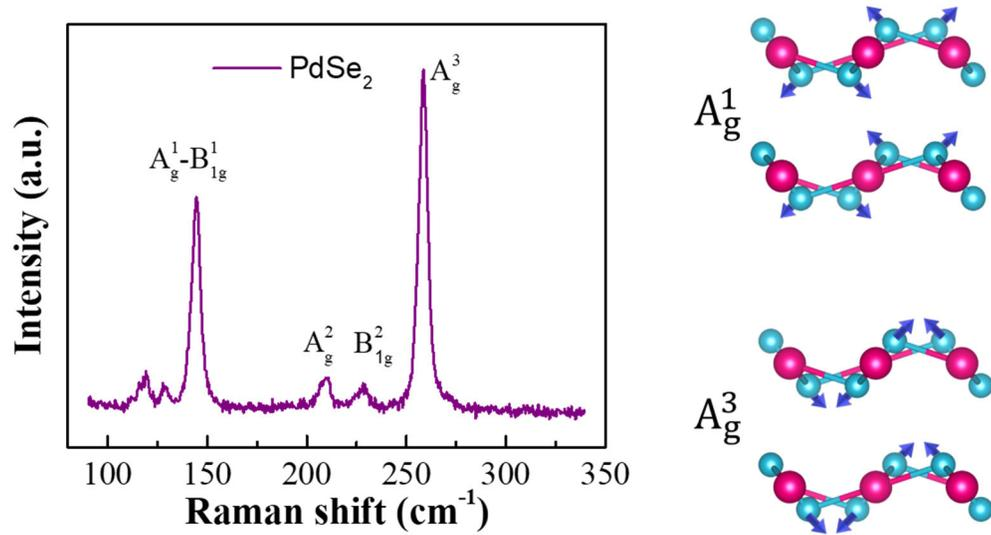
Figure S1. Typical Raman spectra of PdSe<sub>2</sub>. The main peaks in the spectra for bulk structure and Raman-active vibrational modes of  $A_g^1$  and  $A_g^3$ , Red: Pd atom, blue: Se atom.
