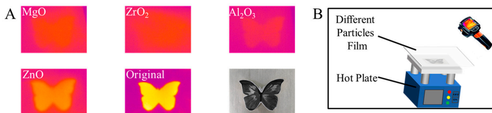
Figure S4 (A). Comparison of IR photos of materials (ZrO 2 , MgO, Al 2 O 3 , ZnO) with the original PP film. They have the same particle size and thickness of the film layer. The IR photo of ZnO in nanoparticles is the clearest and the IR transmission is better. (B). Infrared photo shooting device: the butterfly pattern is placed on the heating table, the film is at a certain height from the heating table, and the position of them (including the film, the heating table and the infrared gun) is the same during each shoot.
