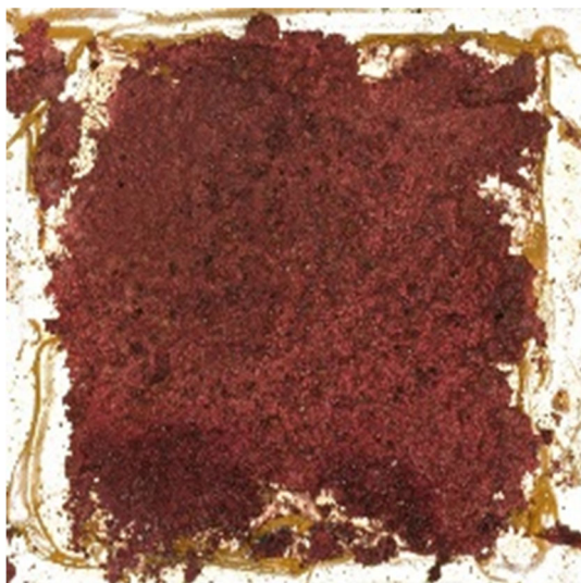
Figure S9. Images of the surfaces of electrodeposited copper layers obtained using electroplating baths without brightening agent.
