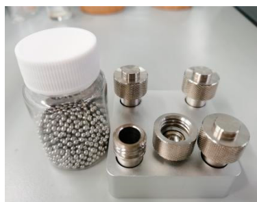
12.0 mm stainless-steel grinding balls and 15 ml stainless-steel milling vessel
