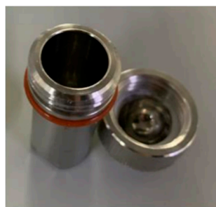
3.0 mm stainless-steel grinding ball and 2 ml stainless-steel milling vessel
