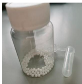
3.0 mm \text{ZrO}_2 grinding balls and 2 ml PP milling tube
