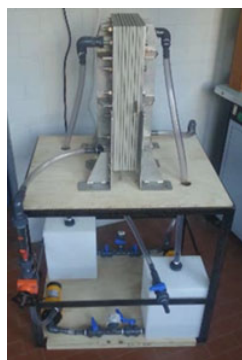
Figure S2. The in-house VRFB five-cell stack.
