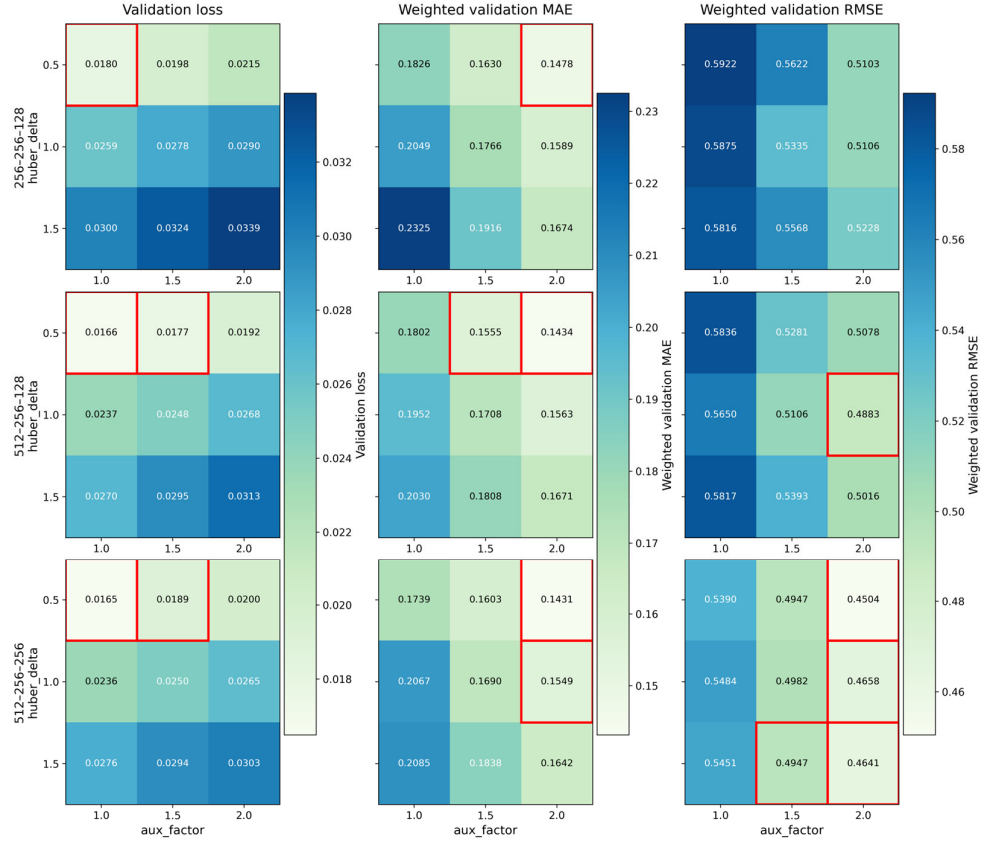
Figure S10. Heatmap summary of the loss-parameter and sample-weighting study (Stage 3). Rows denote the three shortlisted FCNN architectures, and columns denote the reported validation metrics: mean validation loss, mean weighted validation MAE, and mean weighted validation RMSE. Within each panel, rows correspond to the Huber transition threshold \delta and columns to the auxiliary weighting factor. Red outlines highlight the most favorable parameter combinations by metric.
