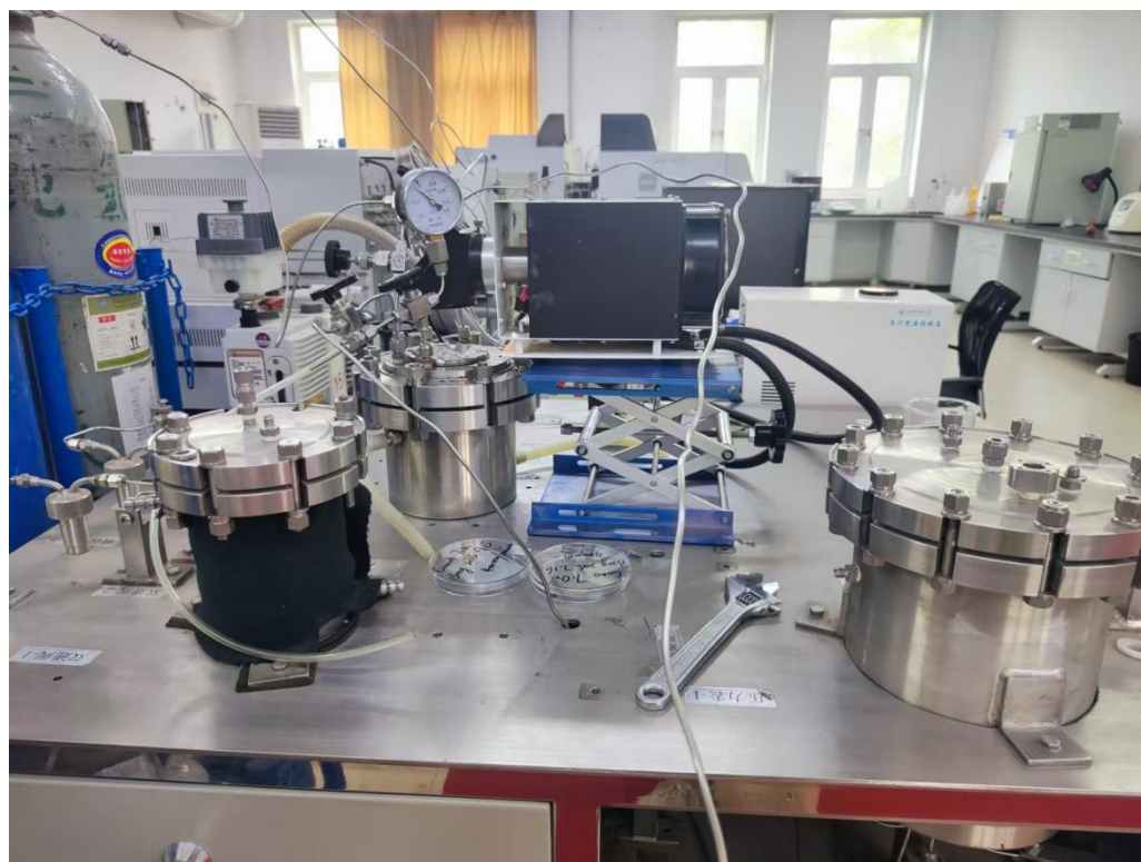
Figure S1. Experimental setup for photocatalytic degradation of gaseous benzene.
