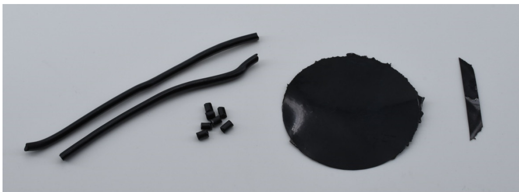
Figure S1. Photos showing the steps of manufacturing the samples: from left to right: extruded strands, pelletized material, compression molded plate, strip cut from the plate and used for the preparation of the sample for TE measurements.
