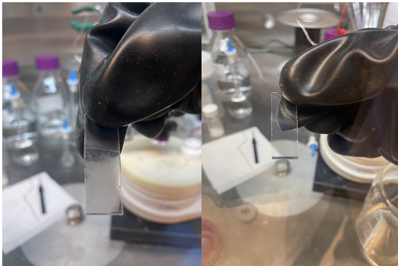
Figure S23: Photographs of FTO working electrode used in diffuse reflectance spectroelectrochemical experiments. The FTO films shown are following: (1) the bulk oxidation and deposition of Pd(dppf)TPT (left), and (2) the subsequent bulk rereduction of the Pd(dppf)TPT -modified film (right).
