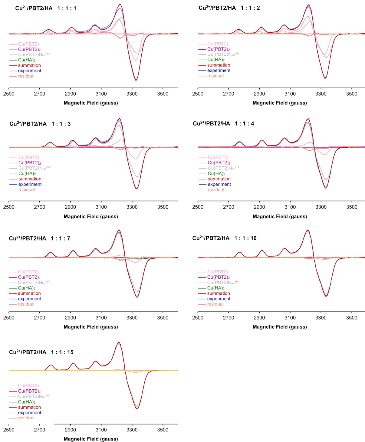
Figure S11. Decomposition of the frozen-solution (77 K) X-band (9.425 GHz) EPR spectra of \text{Cu}/\text{PBT2}/\text{HA} 1 : 1 : n ( n = 1\text{--}15 ). The corresponding percentages of each species are shown in Figure S9c. Blue spectrum , experiment; pink spectrum , \text{Cu}(\text{PBT2}) ; violet spectrum , \text{Cu}(\text{PBT2})_2 ; grey spectrum , \text{Cu}(\text{PBT2})\text{N}_{\text{Im}}^{\text{HA}} ; green spectrum , \text{Cu}(\text{HA})_2 ; red spectrum , summation of \text{Cu}(\text{PBT2}) , \text{Cu}(\text{PBT2})_2 , \text{Cu}(\text{PBT2})\text{N}_{\text{Im}}^{\text{HA}} , and \text{Cu}(\text{HA})_2 spectra; orange spectrum , difference between the experimental spectrum (blue) and the summation (red).
