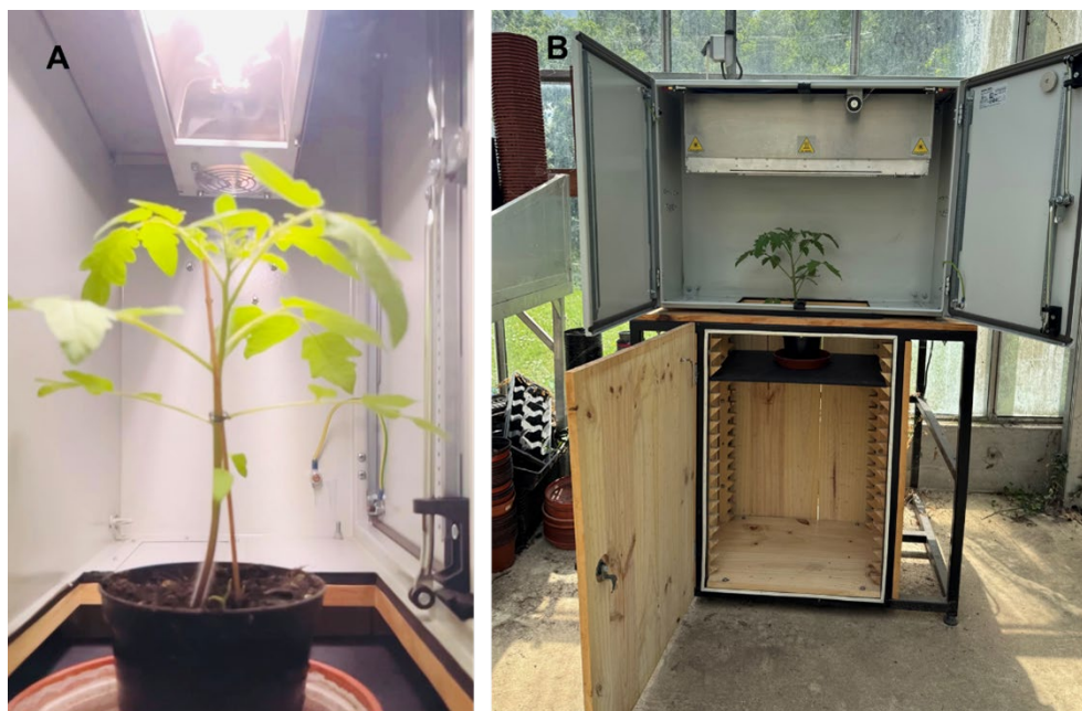
Figure S1: LP.Box system used for pulsed light exposure of tomato plants. A) Initial configuration of the LP.Box showing a tomato plant during light exposure. B) LP.Box mounted on an adjustable support to maintain a constant distance between the upper part of the plant and the light source during growth.
