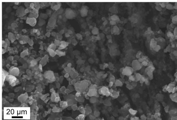
**Figure S4.** SEM micrograph of the  $x = 0.4$  ( $0.6\text{Li}(\text{CB}_9\text{H}_{10})-0.4\text{Li}_2(\text{B}_{12}\text{H}_{12})$ ) compound.
