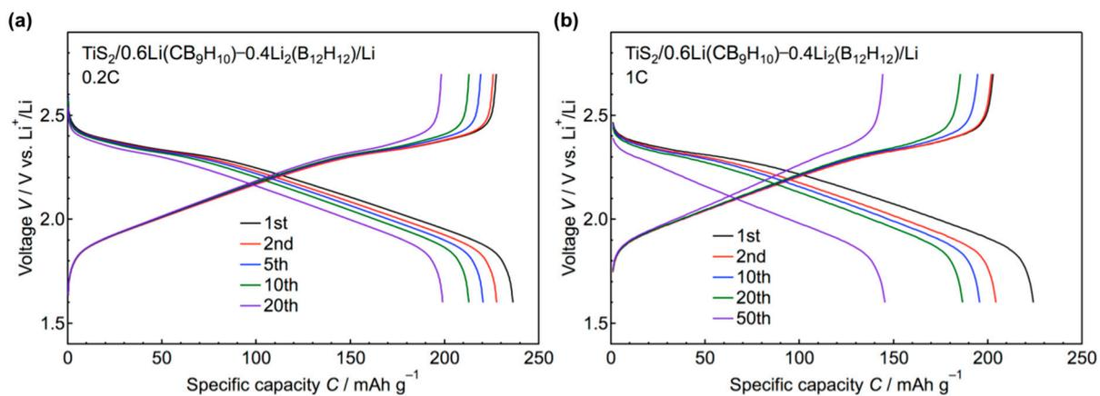
**Figure S7.** Discharge-charge profiles for the TiS<sub>2</sub>/0.6Li(CB<sub>9</sub>H<sub>10</sub>)-0.4Li<sub>2</sub>(B<sub>12</sub>H<sub>12</sub>)/Li cells for rates of (a) 0.2C and (b) 1C.
