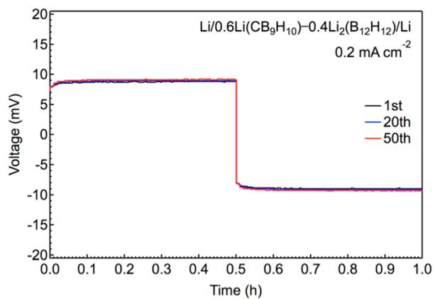
**Figure S6.** Galvanostatic cycling profiles of a Li/0.6Li(CB<sub>9</sub>H<sub>10</sub>)-0.4Li<sub>2</sub>(B<sub>12</sub>H<sub>12</sub>)/Li cell at 0.2 mA cm<sup>-2</sup>.
