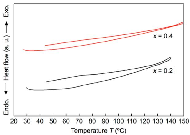
**Figure S2.** Enlarged DTA curves for the  $x = 0.2$  and  $0.4$  compounds in Figure 2.
