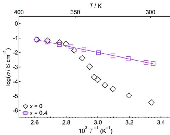
**Figure S3.** Arrhenius plots of the lithium-ion conductivities for the compounds with  $x = 0$  ( $\text{Li}(\text{CB}_9\text{H}_{10})$ ) and  $x = 0.4$  ( $0.6\text{Li}(\text{CB}_9\text{H}_{10})-0.4\text{Li}_2(\text{B}_{12}\text{H}_{12})$ ).
