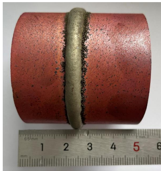
Figure S4. Appearance of single-track Ni60A coating on copper pipe.
