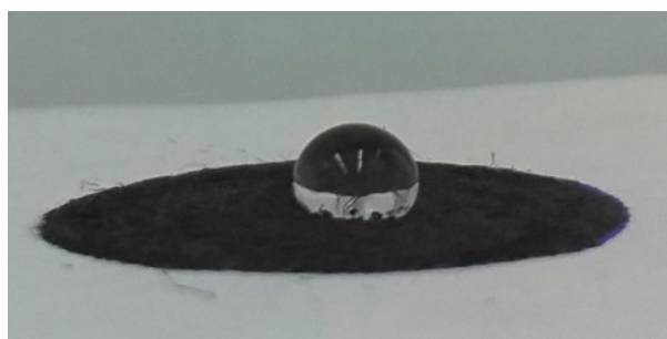
Figure S3. Demonstration of hydrophobicity of pen No 17 on paper No 7 (single side plotting; two passes; pen plotting speed 3.8\text{ cm s}^{-1} ).
