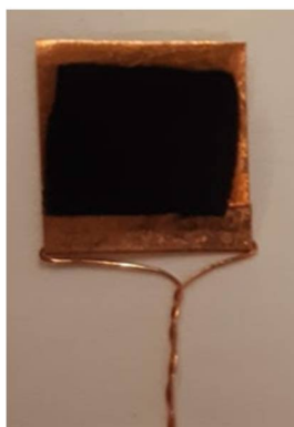
Figure S11. Picture of a carbon foam electrode before being covered by the carbon glue.
