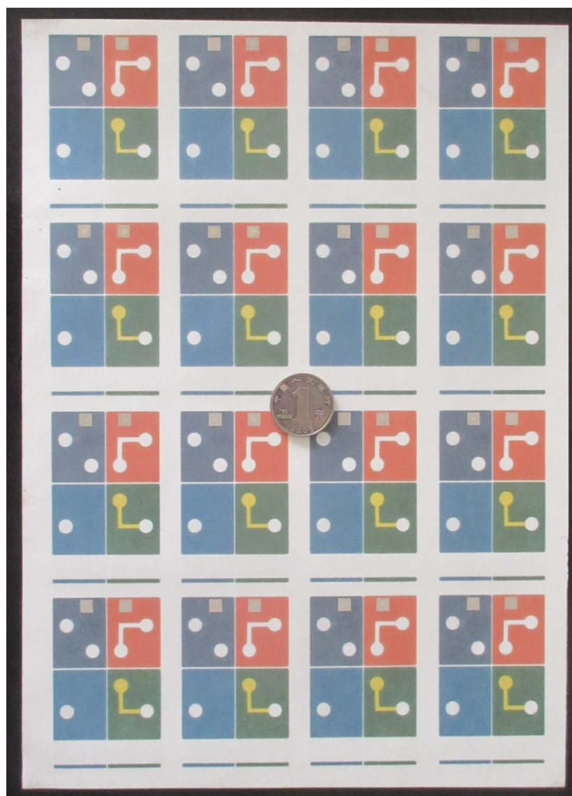
Figure S5. Right side of the 3D- \mu -OBFCAD on a paper sheet (A4) after screen-printing of carbon electrodes, silver wire and drawing of graphite electrodes.
