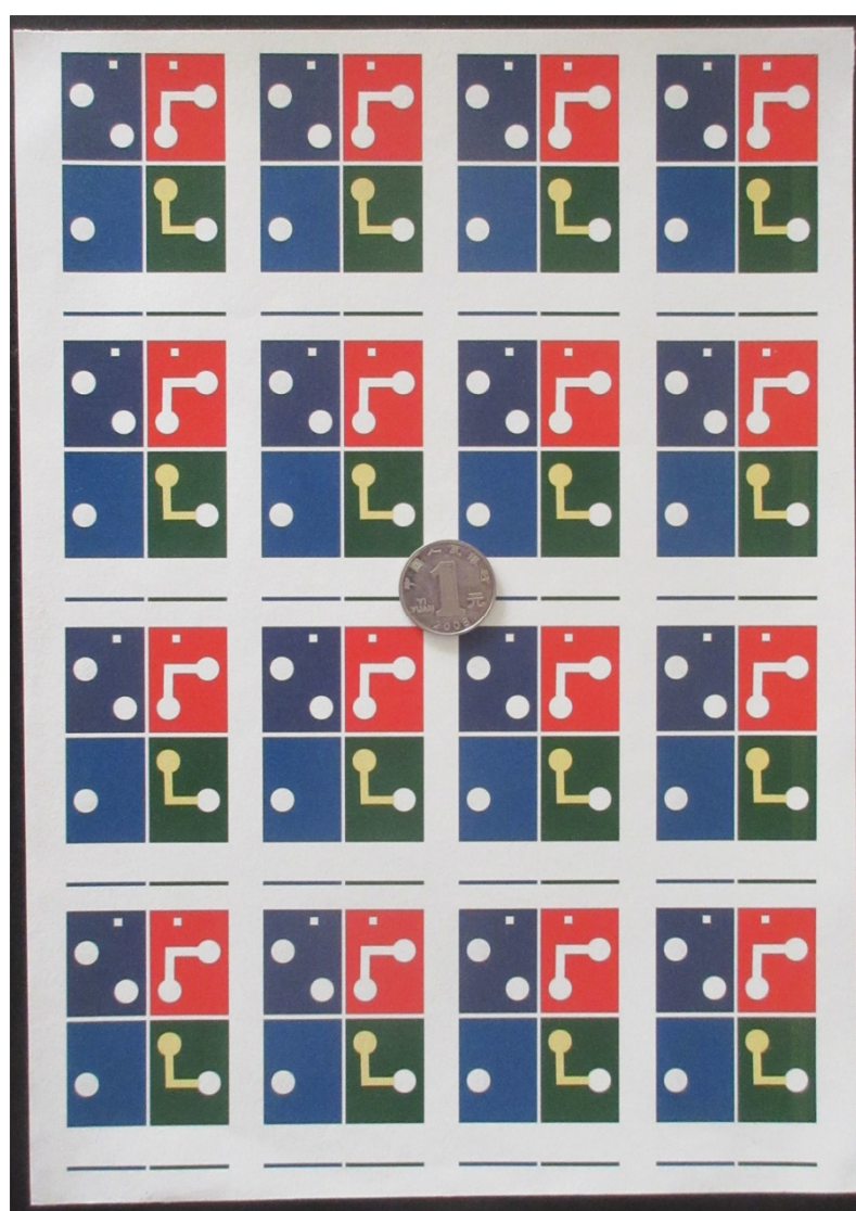
Figure S2. Wax-patterns of 3D- \mu -MOBFCAD on a paper sheet (A4) before baking.
