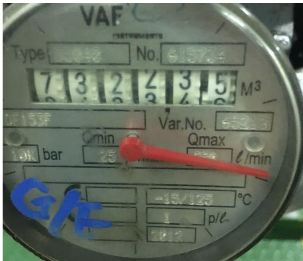
Figure S2 The gauge of measurement of fuel oil consumption on the board
